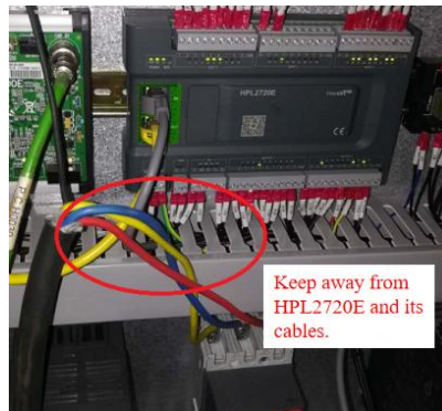
Figure 4-8 Incorrect example: Interference-prone devices not isolated from FSWELD components
