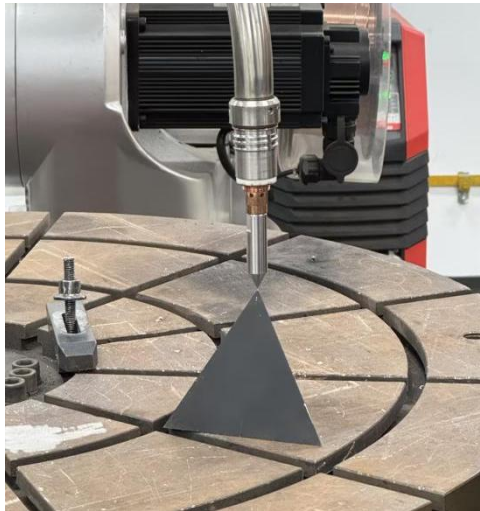
Figure 4-2 Weldgun vertical and tip aligned with calibration point
