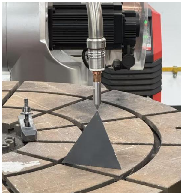
Figure 3-1 Torch vertical and tip aligned with calibration point
