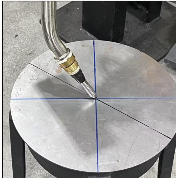
Figure 3-22 Jog the robot arm to make TCP contact the center point
