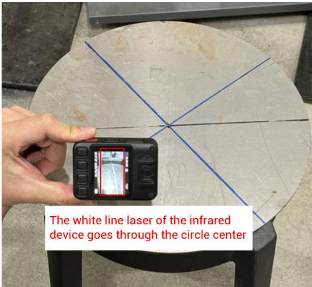
Figure 3-20 Observe line laser position using infrared night vision device
