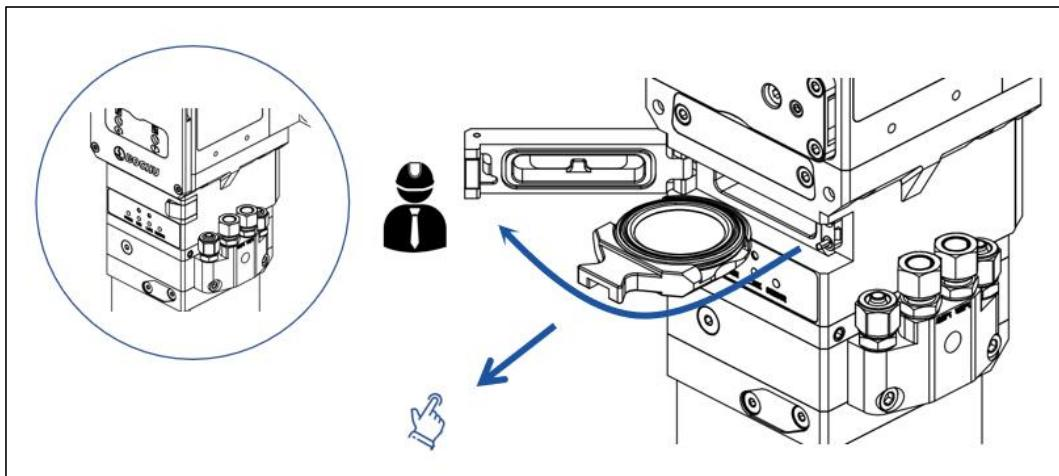
Figure 6-4 Replace the lower protective window
