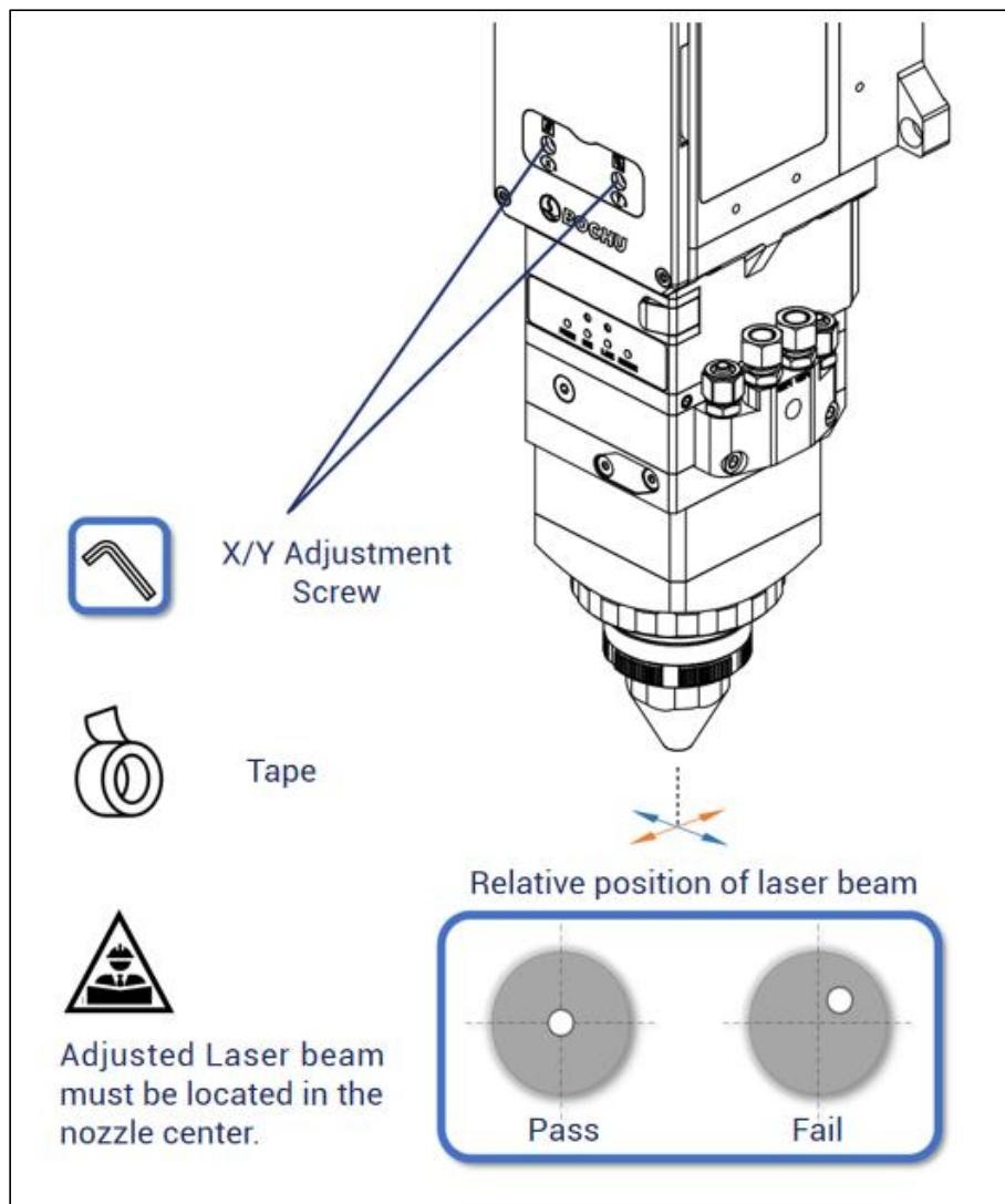
Figure 5-13 Laser beam centering
