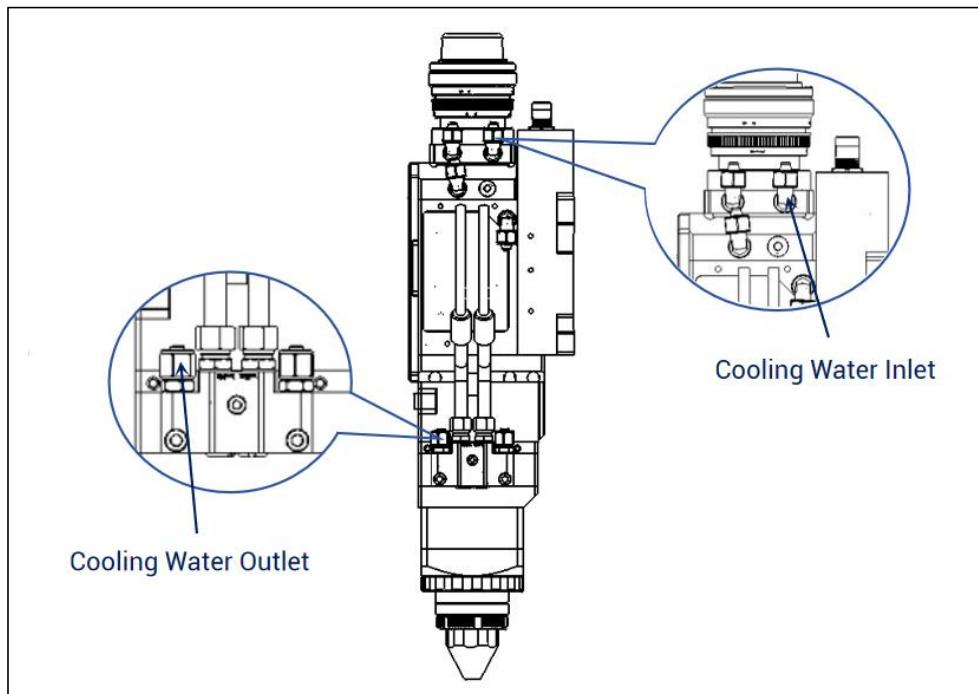
Figure 3-1 Water cooling interfaces
