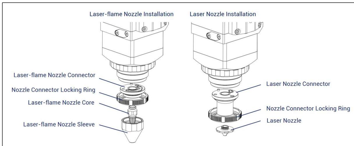
Figure 5-12 Install the nozzle assembly
