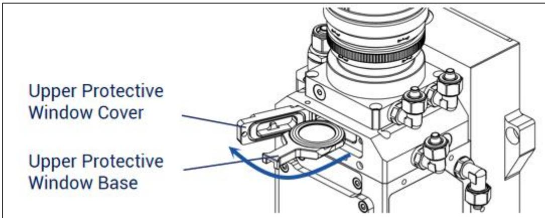
Figure 6-2 Replace the upper protective window
