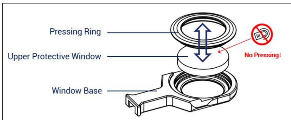
Figure 6-3 Replace the upper protective window
