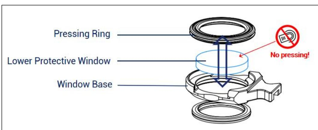
Figure 6-5 Replace the lower protective window
