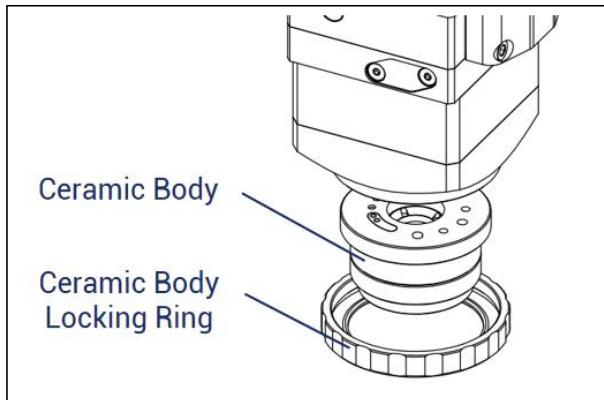
Figure 5-11 Install the ceramic body
