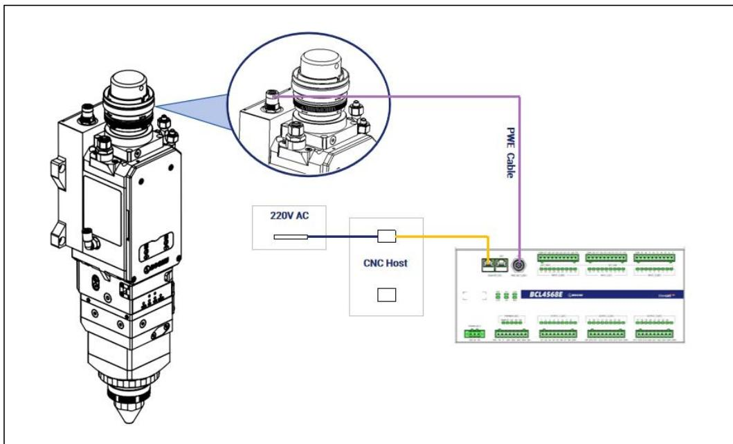
Figure 4-1 Bus system cutting head wiring
