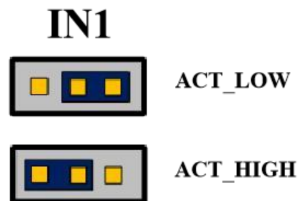
Figure 3-23 IN1 to IN3 adjust the polarity of effective level
