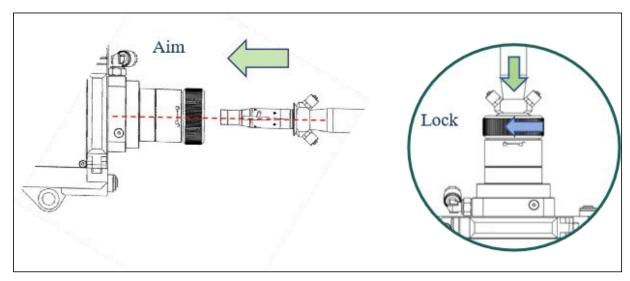
Figure 5-5 Insert the laser fiber connector
