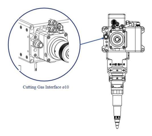
Figure 2-1 Cutting gas interface
