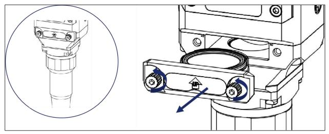
Figure 6-4 Replace the lower protective window
