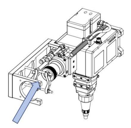
Figure 5-11 Insert the laser connector
