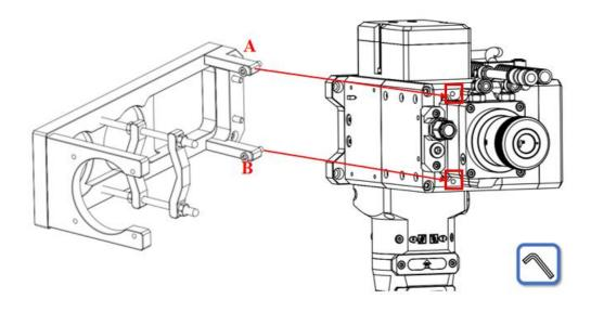
Figure 5-10 Attach the laser clamping unit
