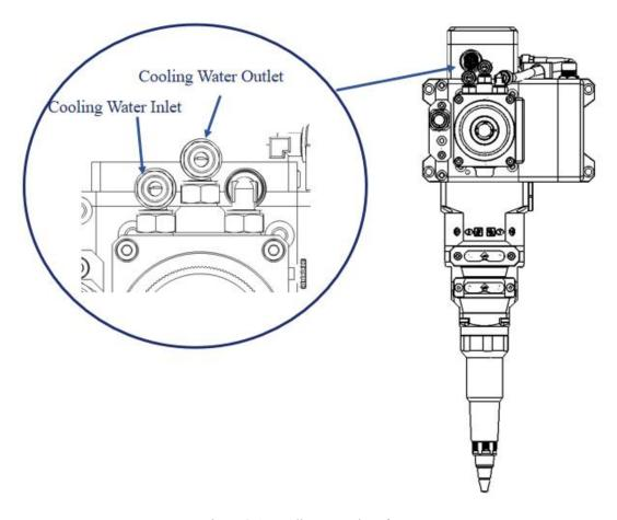
Figure 3-1 Cooling water interfaces
