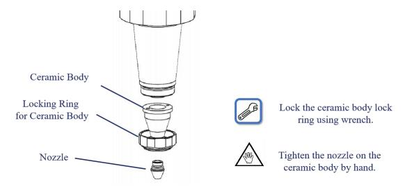
Figure 5-8 Ceramic body and nozzle installation
