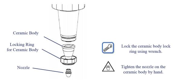
Figure 5-8 Ceramic body and nozzle installation
