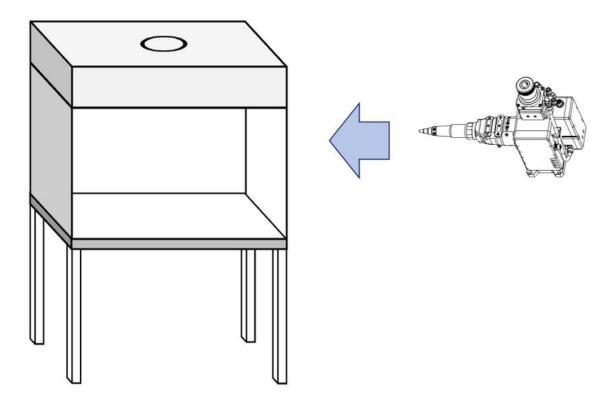
Figure 5-3 Put the cutting head inside the workbench
