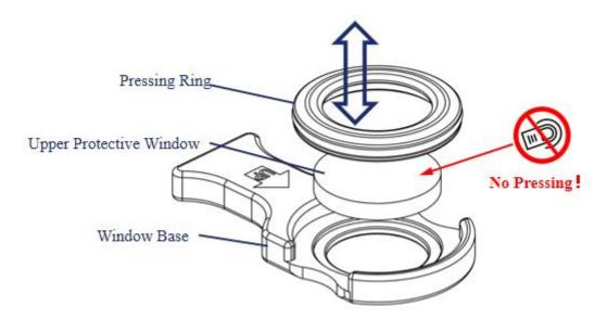
Figure 6-3 Insert the window cartridge
