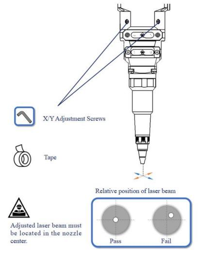
Figure 5-9 Laser beam centering
