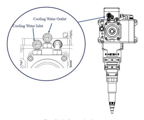
Figure 3-1 Cooling water interfaces
