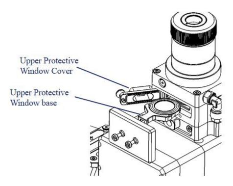
Figure 6-2 Replace the 1st upper protective window
