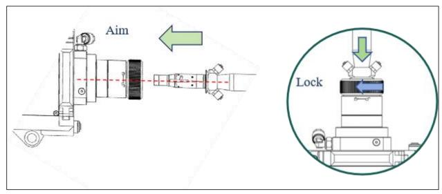
Figure 5-5 Insert the laser fiber connector
