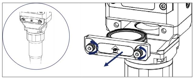
Figure 6-4 Replace the lower protective window
