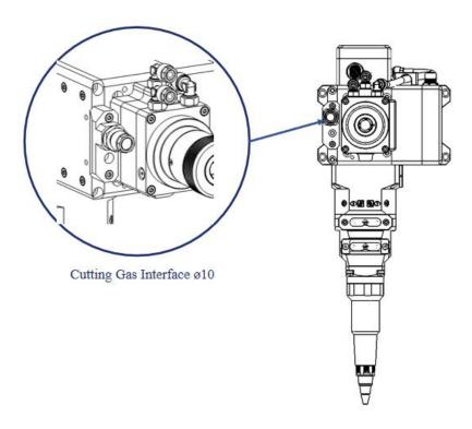
Figure 2-1 Cutting gas interface
