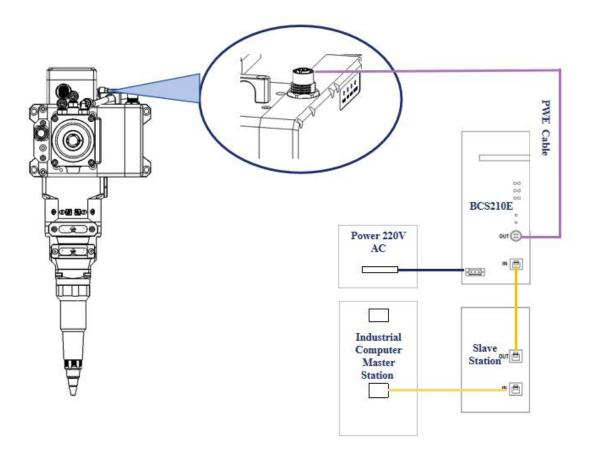
Figure 4-1 Bus system wiring diagram
