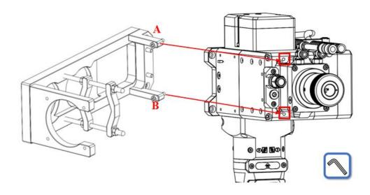
Figure 5-10 Attach the laser clamping unit
