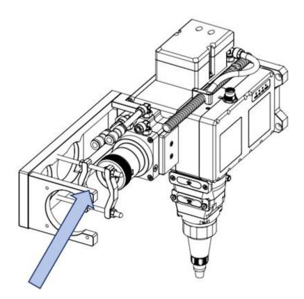
Figure 5-11 Insert the laser connector
