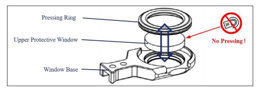
Figure 6-3 Insert the window cartridge
