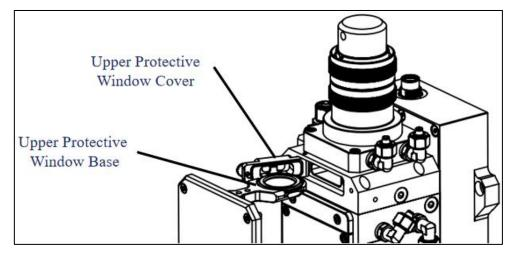
Figure 6-2 Replace the 1st upper protective window
