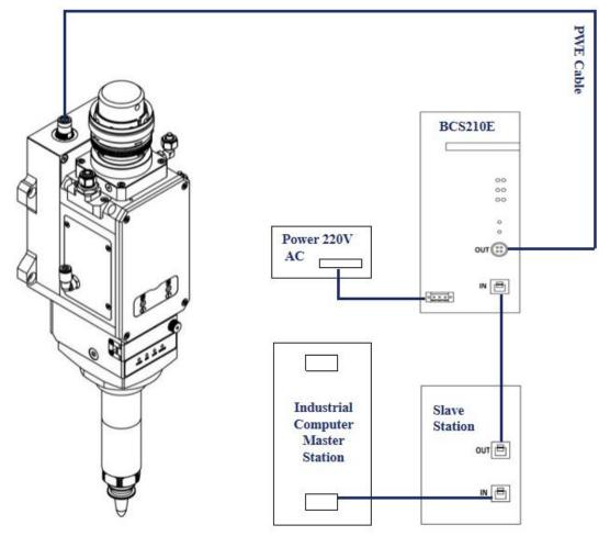
Figure 4-1 Bus system wiring diagram
