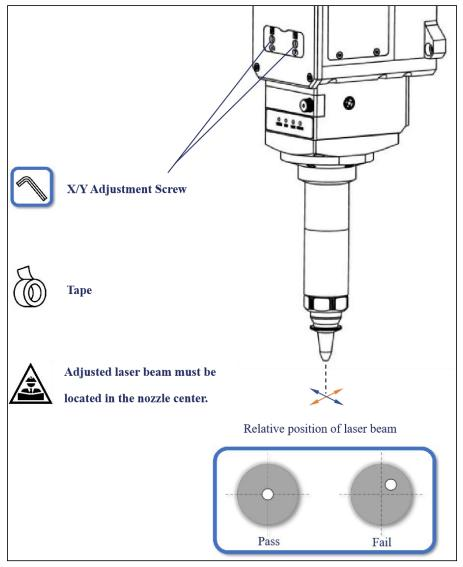
Figure 5-10 Laser beam centering
