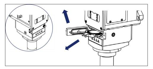
Figure 6-4 Replace the lower protective window
