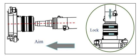
Figure 5-6 Insert the laser fiber connector
