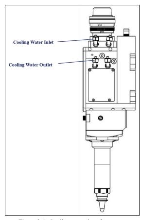
Figure 3-1 Cooling water interfaces
