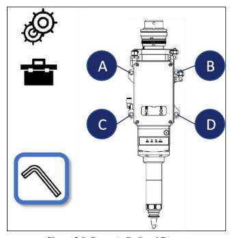
Figure 5-8 Screw A, B, C and D
