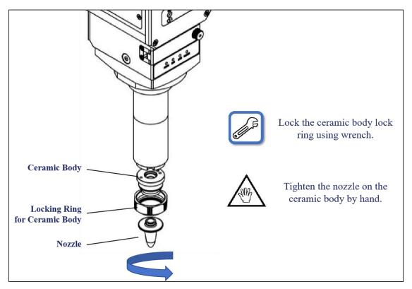
Figure 5-9 Ceramic body and nozzle installation
