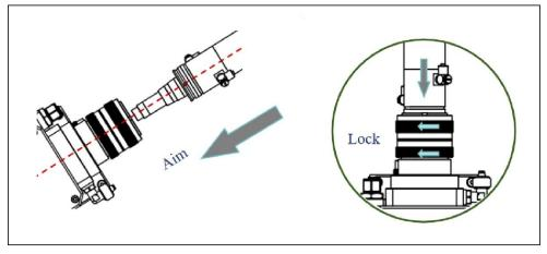
Figure 5-6 Insert the laser fiber connector
