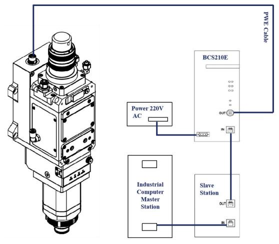
Figure 4-1 Bus system wiring diagram
