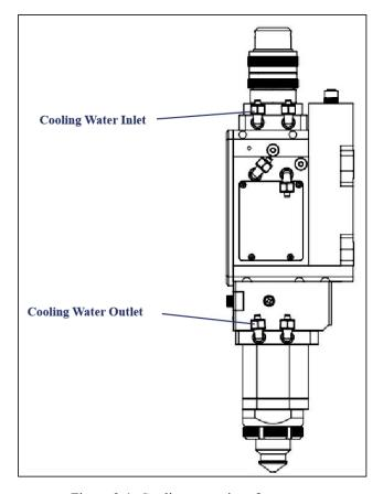
Figure 3-1 Cooling water interfaces
