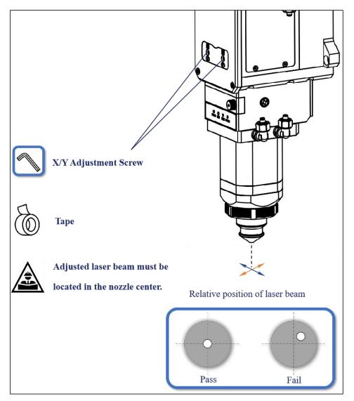
Figure 5-10 Laser beam centering
