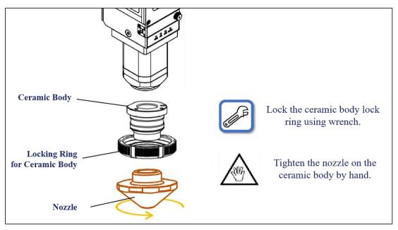
Figure 5-9 Ceramic body and nozzle installation
