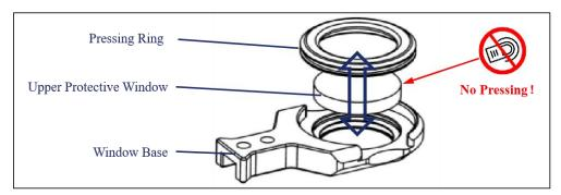
Figure 6-3 Insert the window cartridge
