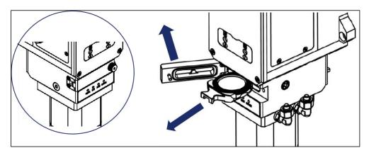
Figure 6-4 Replace the lower protective window
