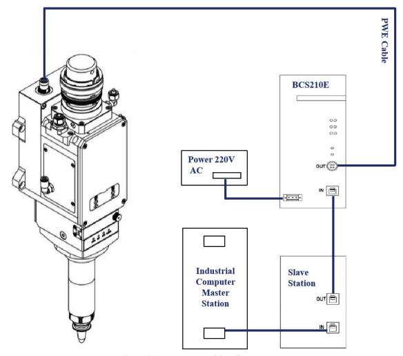
Figure 4-1 Bus system wiring diagram
