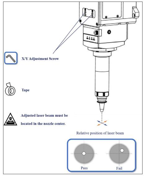
Figure 5-10 Laser beam centering
