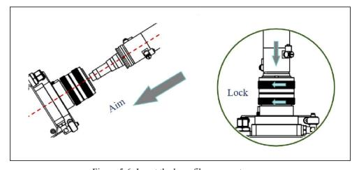
Figure 5-6 Insert the laser fiber connector
