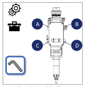
Figure 5-8 Screw A, B, C and D
