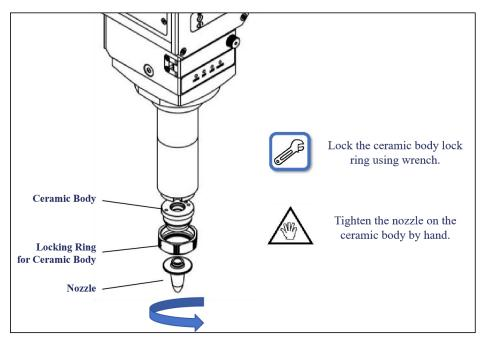
Figure 5-9 Ceramic body and nozzle installation
