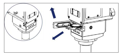
Figure 6-4 Replace the lower protective window
