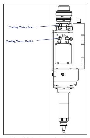
Figure 3-1 Cooling water interfaces
