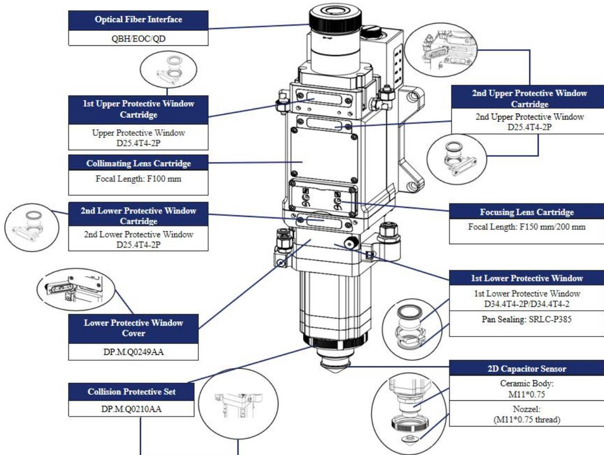
Figure 6-1 Product structure diagram
