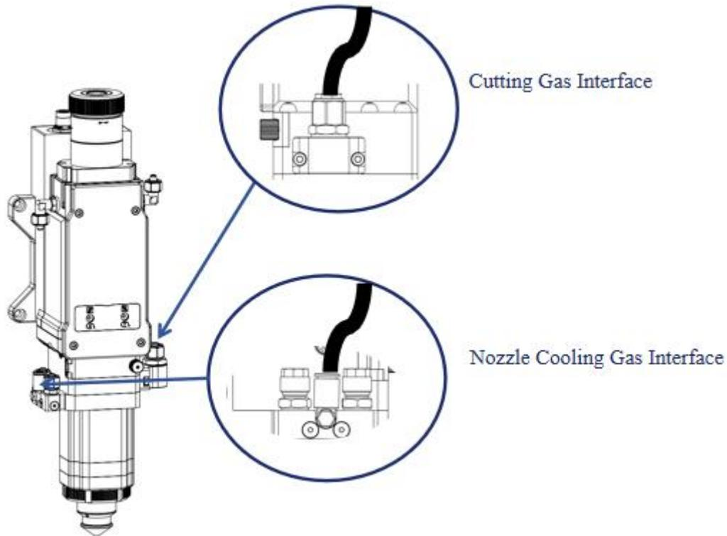
Figure 2-1 Installation connection: Cutting gas
