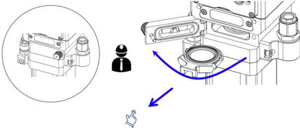
Figure 6-4 Change the lower protective window
