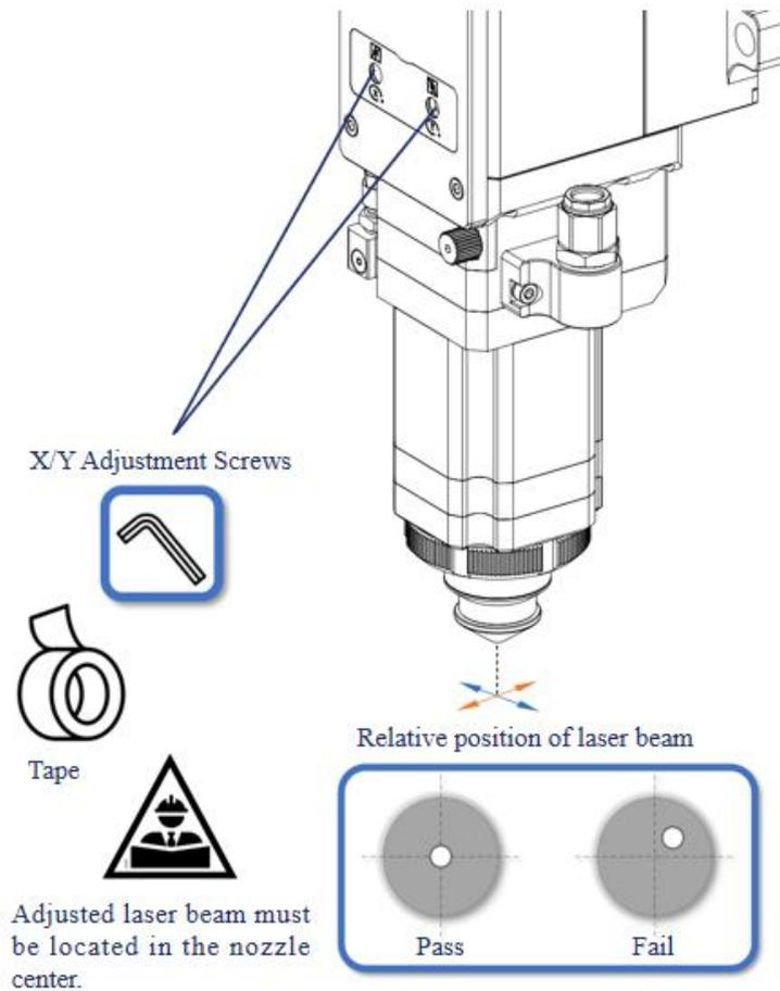
Figure 5-9 Laser beam centering
