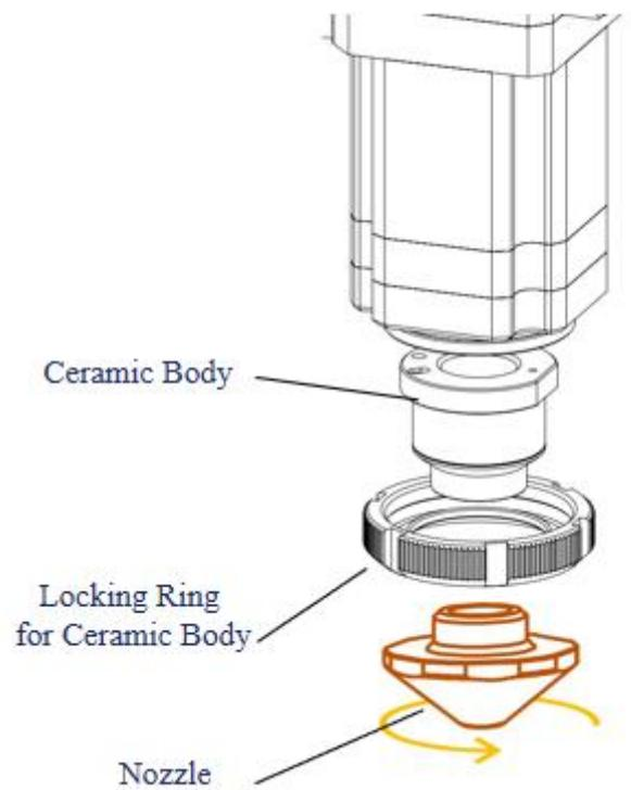
Figure 5-8 Ceramic body and nozzle
