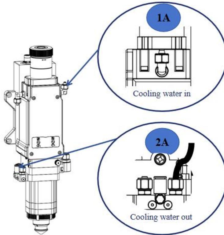
Figure 3-1 Cooling water interface: Inlet 1A, Outlet 2A.
