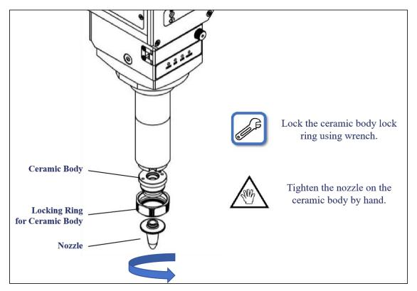
Figure 5-9 Ceramic body and nozzle installation
