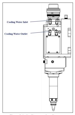
Figure 3-1 Cooling water interfaces
