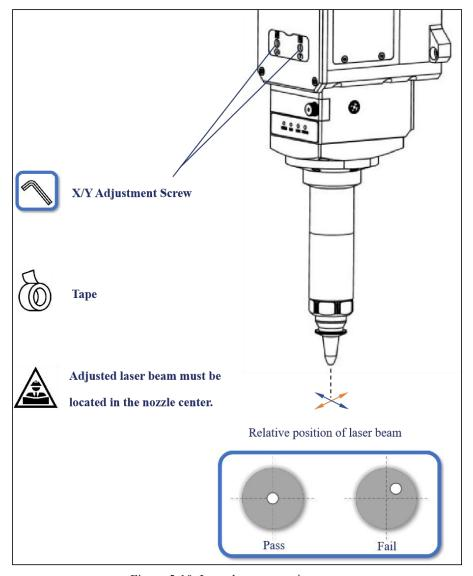
Figure 5-10 Laser beam centering
