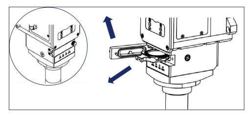
Figure 6-4 Replace the lower protective window
