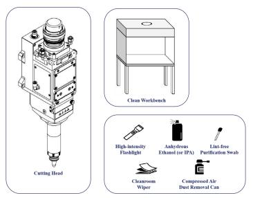
Figure 5-1 Preparation tools for the cutting head installation
