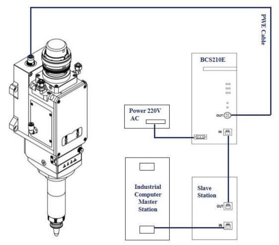
Figure 4-1 Bus system wiring diagram
