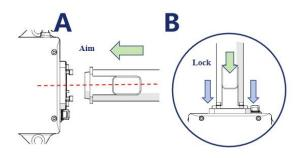
Figure 6-8 Insert the ADD fiber connector
