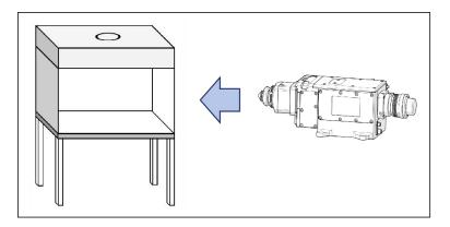
Figure 6-3 Put the cutting head inside the workbench
