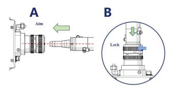
Figure 6-6 Insert the QD fiber connector
