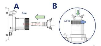
Figure 6-5 Insert the QBH fiber connector
