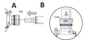
Figure 6-7 Insert the Q+ fiber connector
