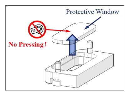
Figure 7-9 Take out the contaminated window
