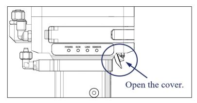
Figure 7-7 Open the cover plate
