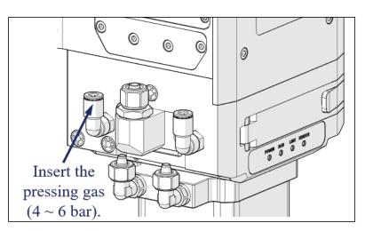
Figure 7-6 Insert gas (4~6 bar)
