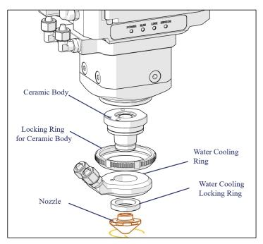
Figure 6-14 Ceramic body and nozzle
