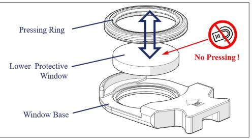
Figure 7-5 Insert window cartridge
