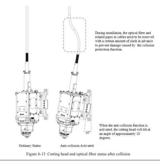
Caution: When the anti-collision backplate is optionally equipped, the cutting head will tilt to a certain extent (less than 10°) when it is impacted. In order to avoid damaging the optical fiber, the optical fiber must be reserved with a slack of more than 100 mm, and the distance between the fixed point of the optical fiber and the end of the optical fiber cable should be ensured to be more than 270 mm.
