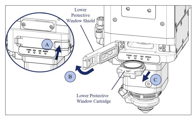
Figure 7-4 Change the lower protective window
