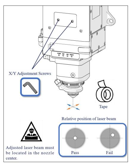
Figure 6-15 Laser beam centering
