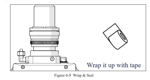
Caution: To ensure a proper seal, it is recommended to wrap at least three layers of tape for sealing.
