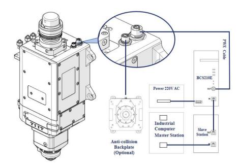
The electrical connections of the cutting head are shown in the figure below:
