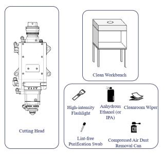
Figure 6-1 Preparation tools for the cutting head installation
