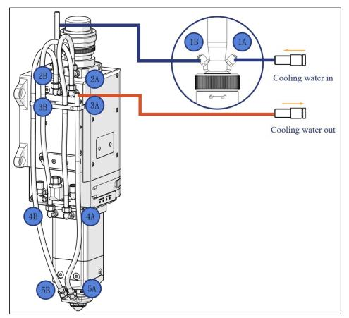
Figure 3-1 Cooling water interfaces
