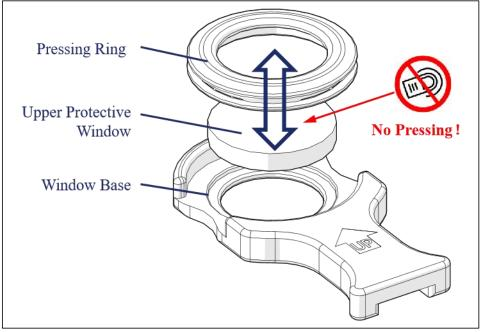
Figure 7-3 Insert window cartridge
