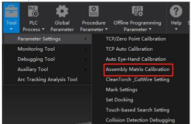
Before calibration, ensure that the TCP calibration error of the robotic arm is within 2mm. Place a marker at a fixed position, which can be a cone or a triangular prism. Point the TCP to the marker and record the coordinates. Move the external axis by more than 100 mm, point the TCP to the marker again, and record the coordinates to complete the calibration.
