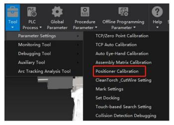
The software will automatically recognize the current scene and display different calibration interfaces based on whether it's a fixed worktable, single-axis positioner, or double-axis positioner.
