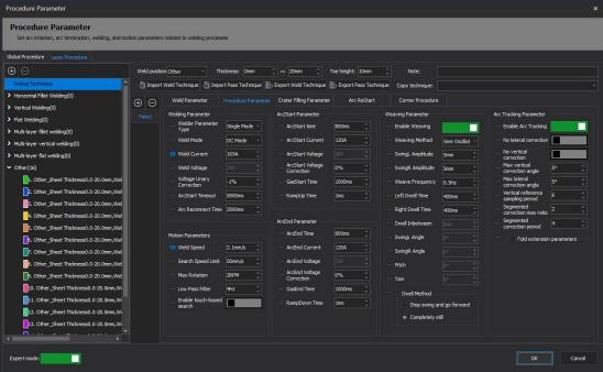
Set the process match table according to the actual requirements, such as plate thickness range, welding position, and bevel angle.
