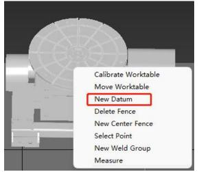
Move the TCP to three different positions on the fence surface, ensuring a significant height difference in the Z-direction, and record the coordinates. The fence needs to calibrate two mutually perpendicular fence surfaces.
