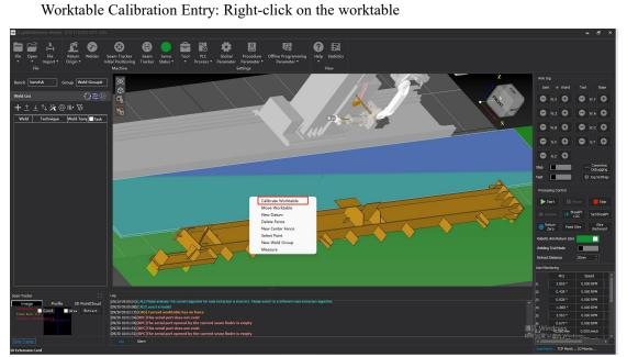
By default, a fixed worktable is a complete plane. Use the robotic arm's TCP to touch three different positions on the worktable surface and record the coordinates; the three points should be as far apart as possible. For ground rail with jig, please ensure that the three marker positions are on the same horizontal plane.
