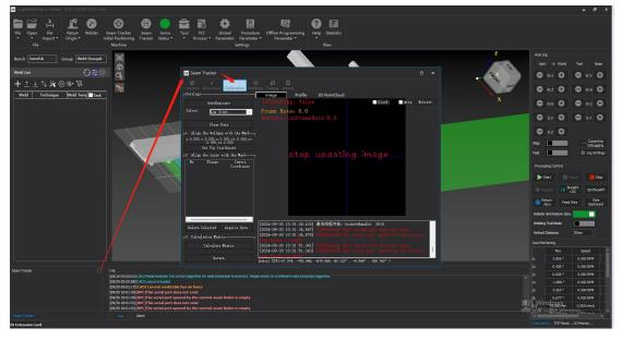
Before calibration, keep the lower surface of the camera parallel to the ground. Prepare calibration sample templates in advance; options include a triangular prism or a step piece. Before hand-eye calibration, please make sure the TCP calibration error of the robotic arm is within 2mm. The BCW600P camera has two viewing distances: near and far. Please calibrate for each separately.
