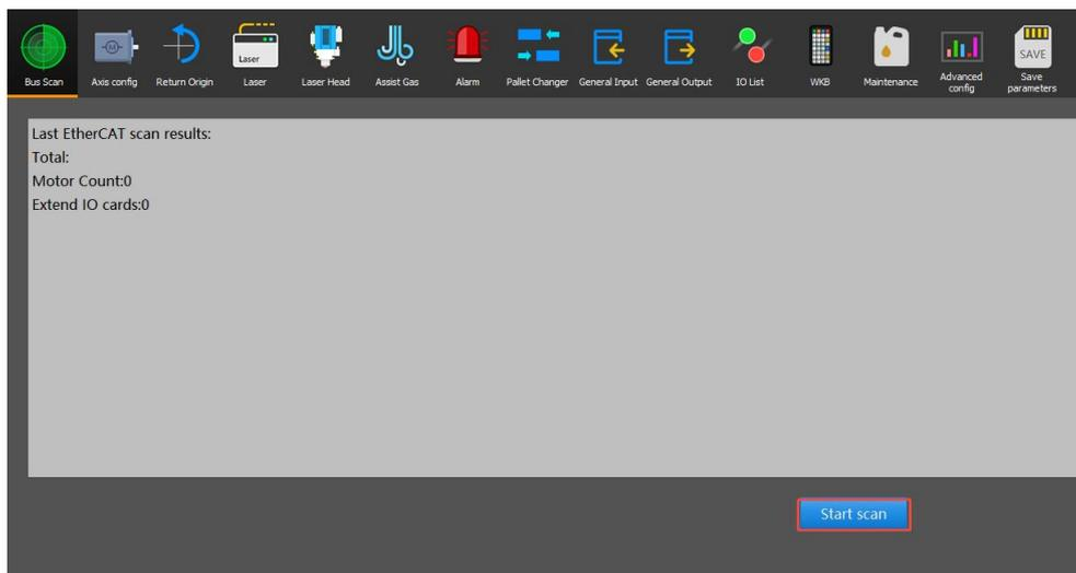
Figure 7-6 Scan the connected slave
