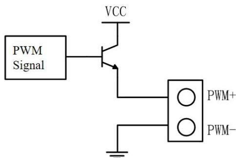
Figure 4-5 PWM output circuit
