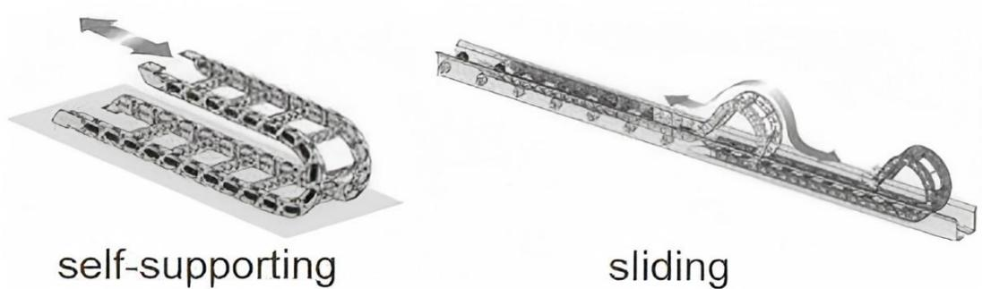
Figure 8-2 Self-Supporting and sliding
