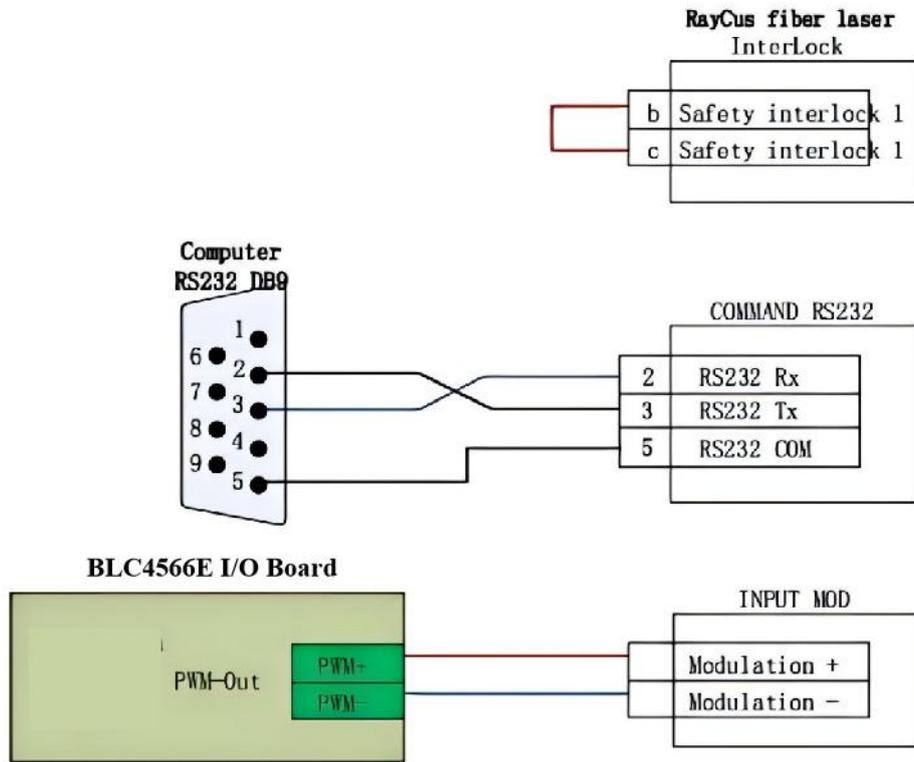
Figure 6-3 RayCus laser wiring
