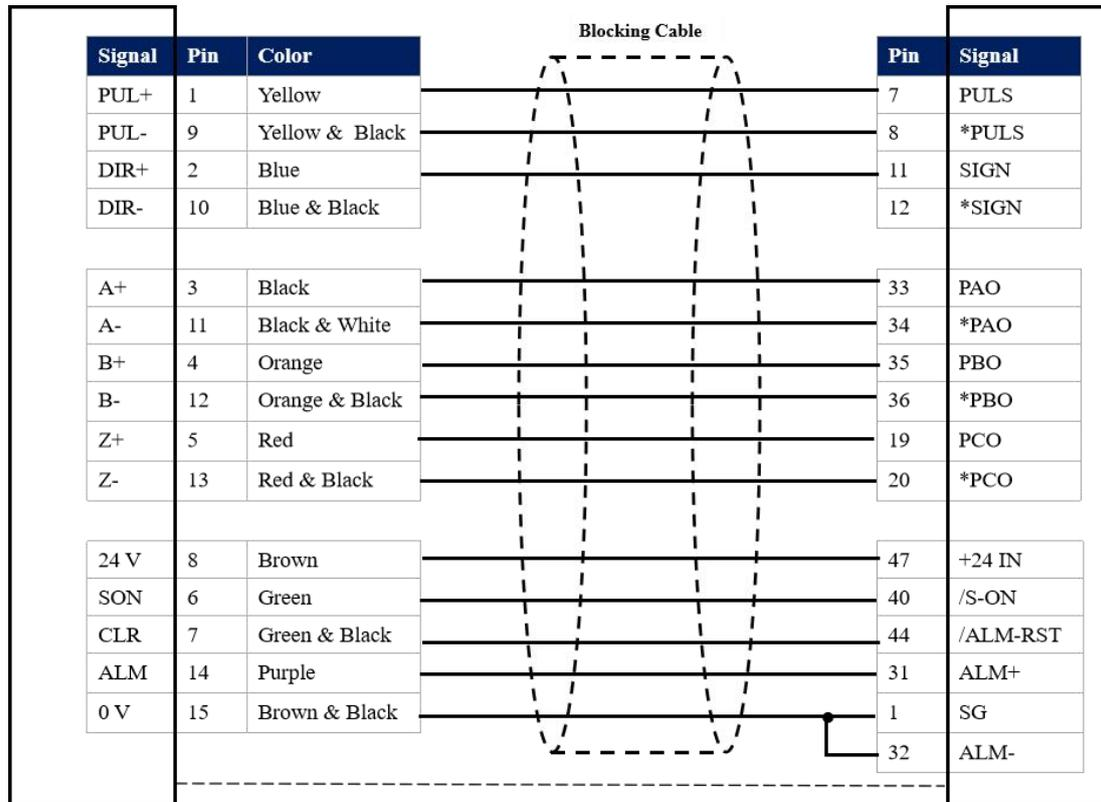
Figure 4-14 Axis wiring diagram for Yaskawa servo
