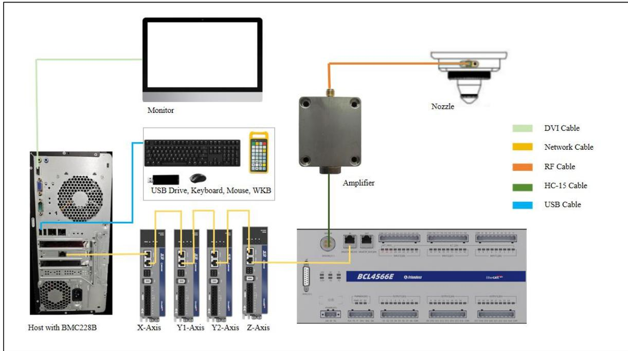
Figure 1-2 System wiring for Non-BLT cutting head
