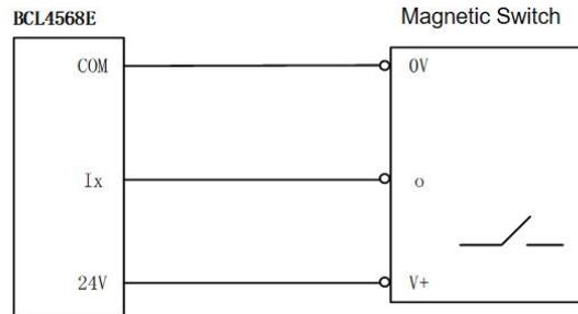
Figure 3-11 Magnetic Switch wiring
