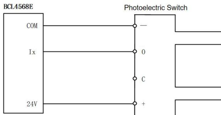
Figure 3-9 Photoelectric Switch wiring
