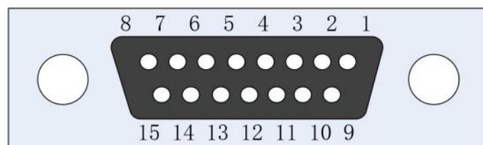
Figure 4-13 Servo driver interfaces
