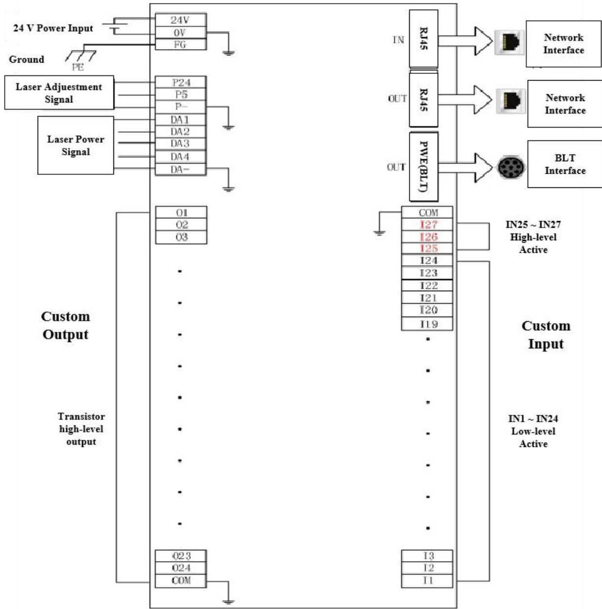
Figure 3-15 BCL4568E wiring
