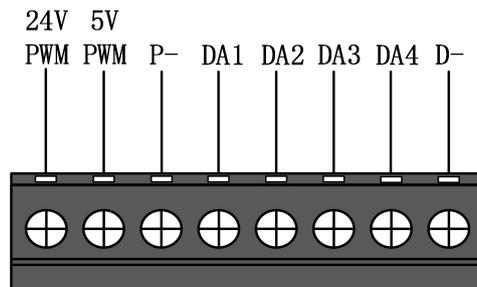
Figure 4-4 PWM/DA wiring terminal
