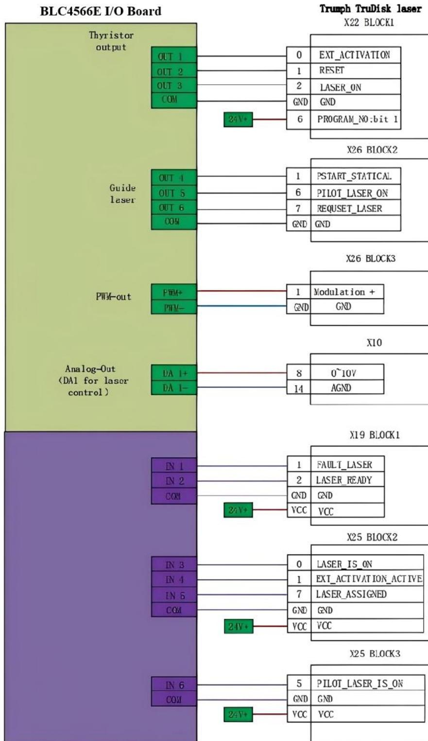
Figure 6-4 Trumpf laser wiring
