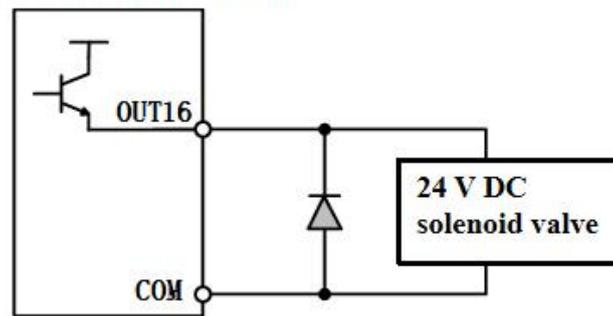
Figure 8-3 Connect a freewheeling diode in parallel at both ends of the Solenoid Valve
