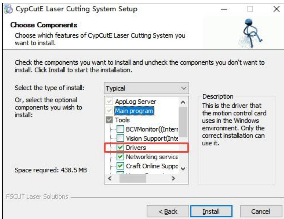
Figure 7-1 Install drivers during CypCutE installation
