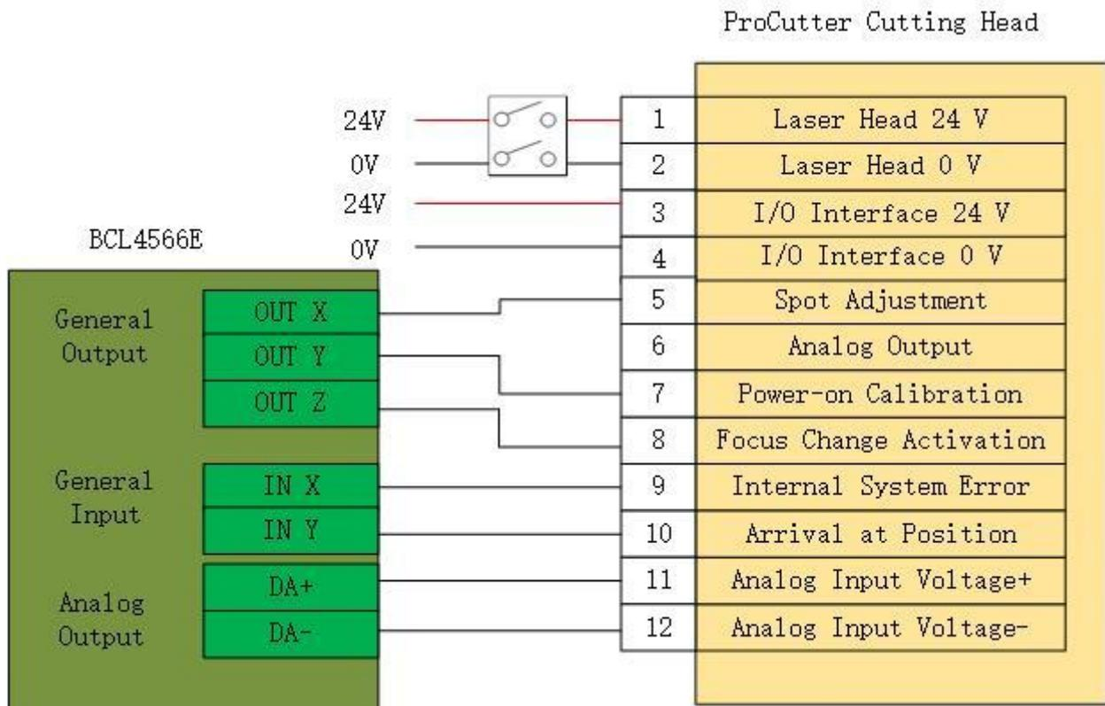
Figure 5-1 ProCutter wiring
