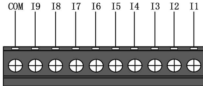
Figure 4-7 Input wiring terminals
