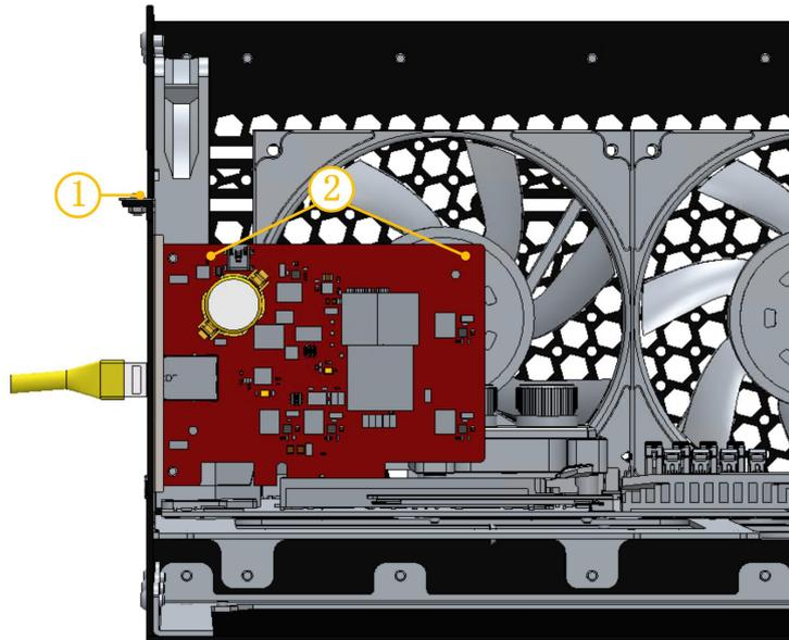
Figure 2-3 BMC228B control card installation
