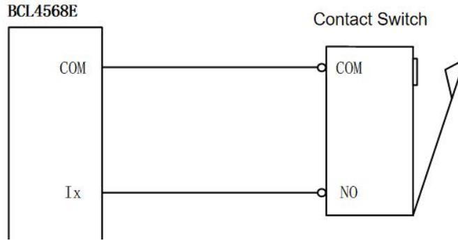
Figure 3-10 Contact Switch wiring
