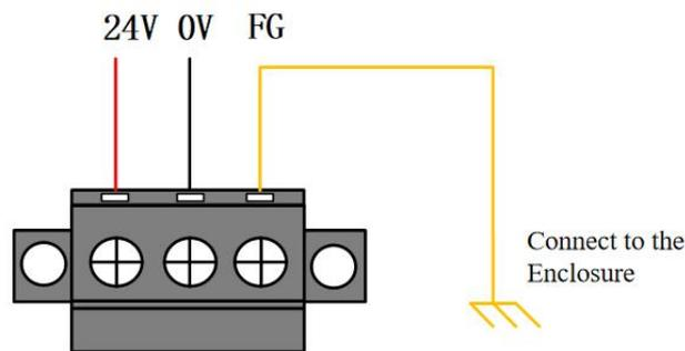
Figure 4-3 Power wiring terminals
