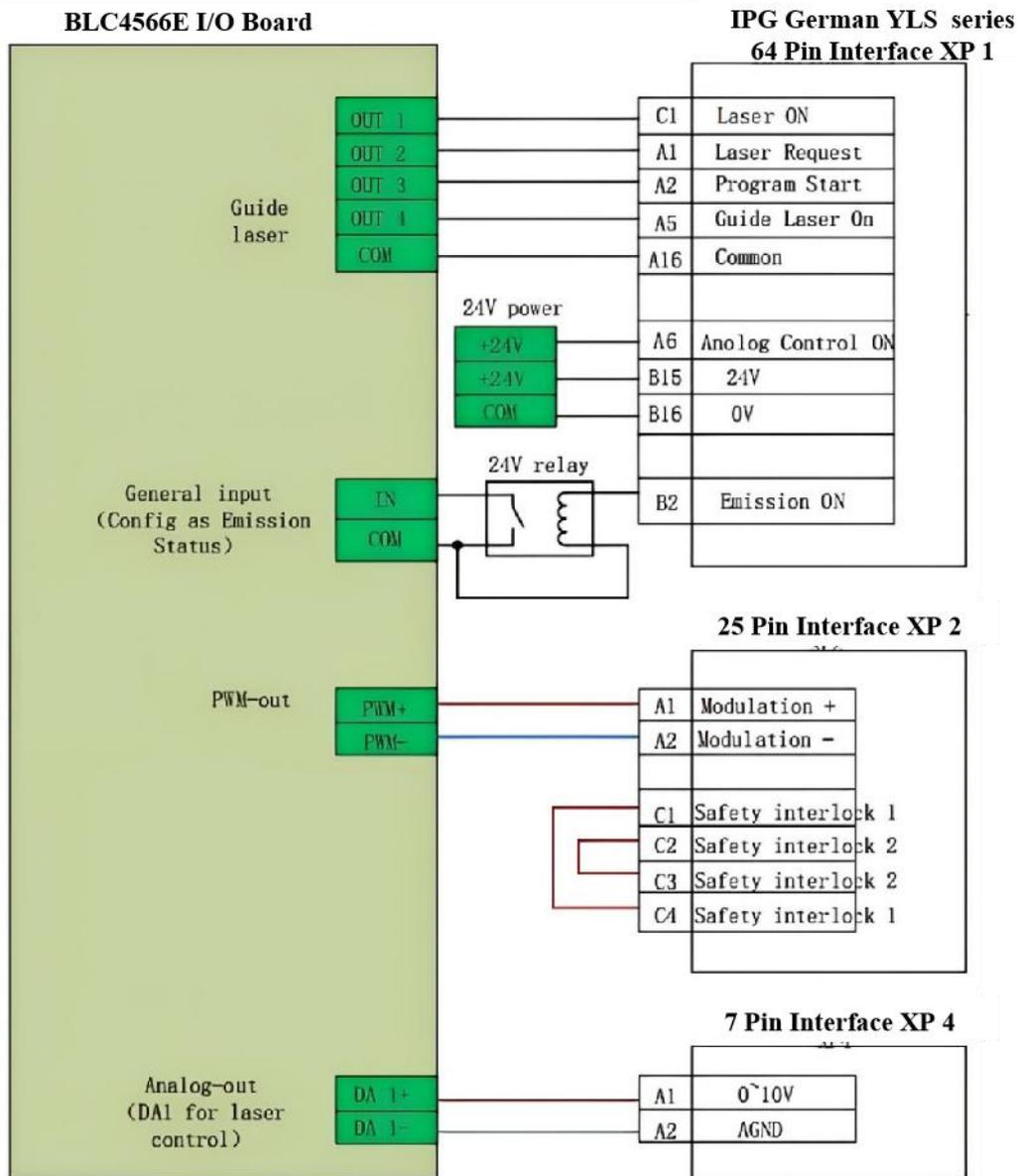
Figure 6-1 IPG-German laser wiring
