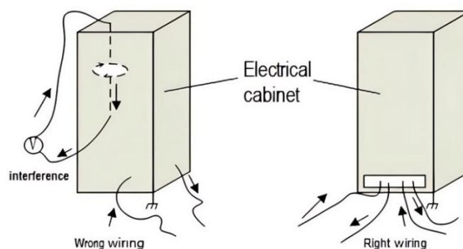
Figure 8-4 Cabinet wiring
