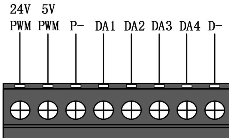
Figure 3-5 PWM/DA wiring terminal
