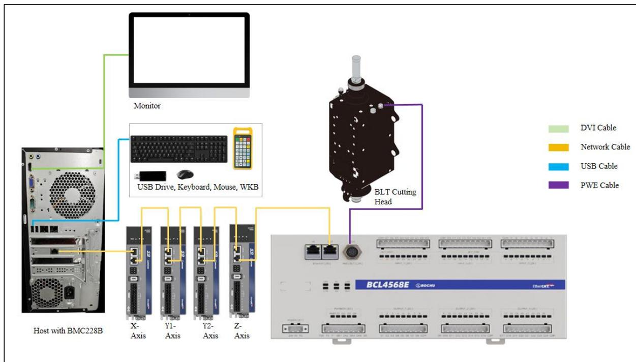
Figure 1-1 System wiring for BLT cutting head
