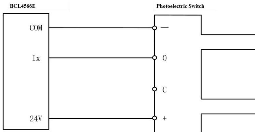
Figure 4-8 Photoelectric switch wiring
