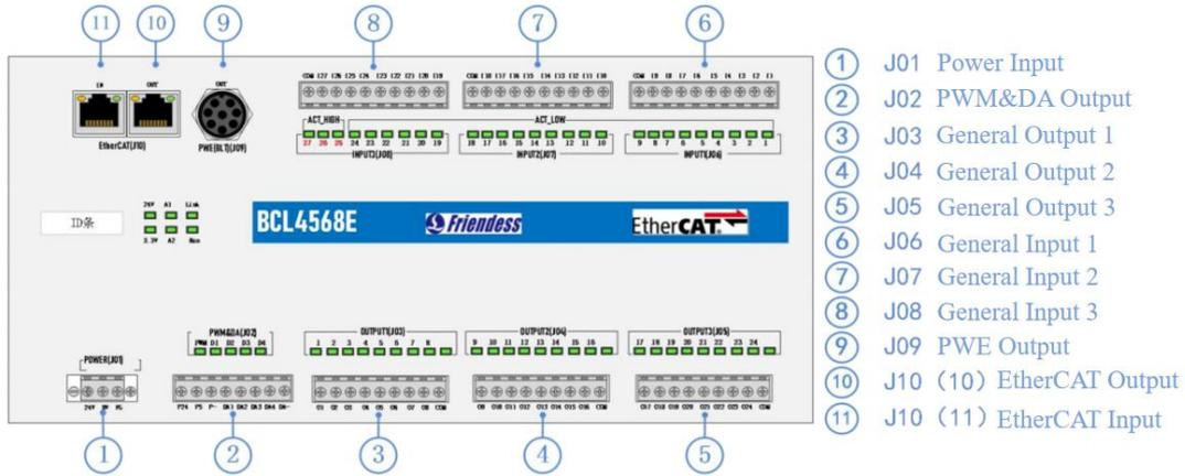
Figure 3-3 Detailed interface layout of BCL4568E terminal
