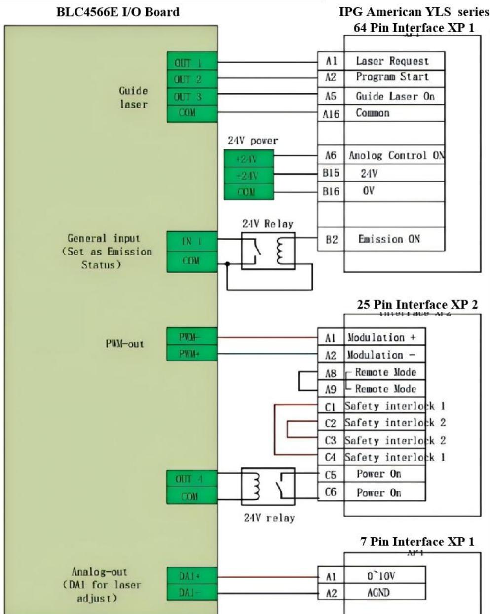
Figure 6-2 IPG-American laser wiring
