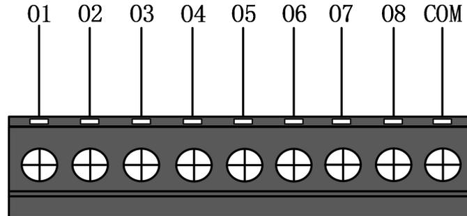
Figure 4-6 Output wiring terminals
