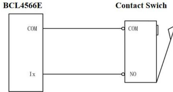
Figure 4-9 Contact switch wiring
