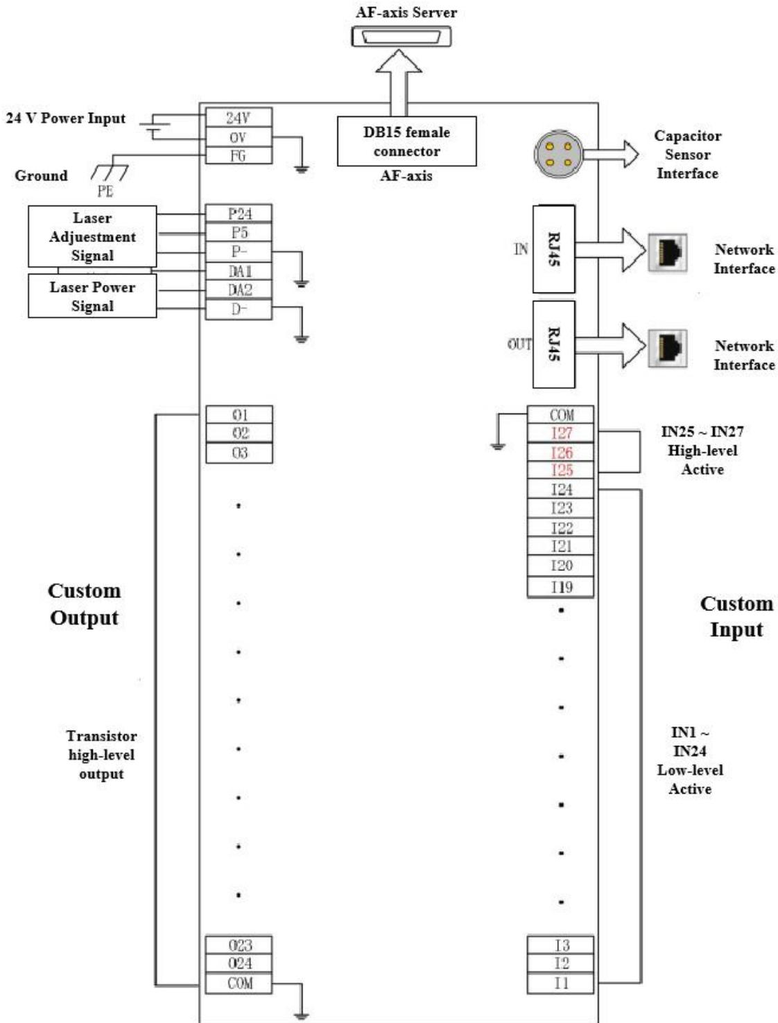
Figure 4-15 BCL4566E wiring
