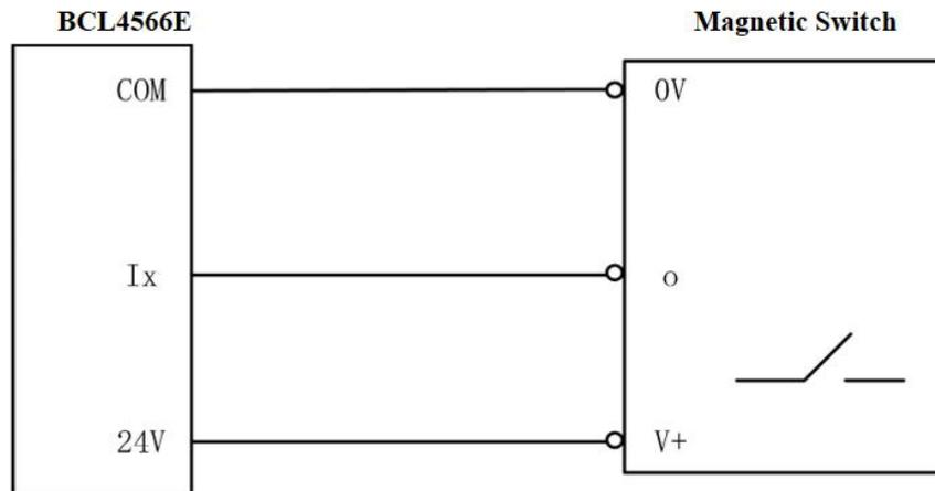
Figure 4-10 Magnetic switch wiring
