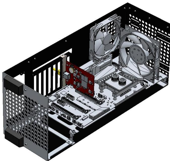
Figure 2-4 BMC228B control card after installation
