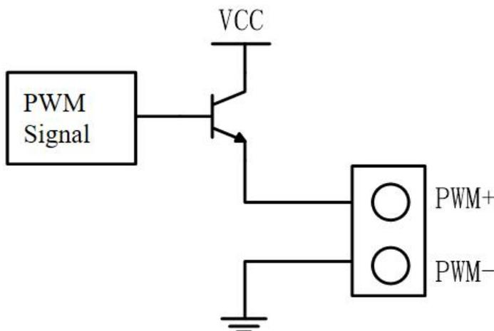
Figure 3-6 PWM output circuit
