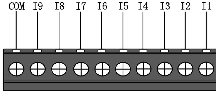
Figure 3-8 Input wiring terminals
