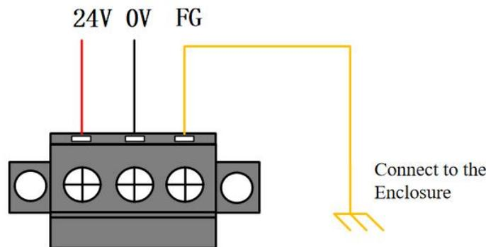
Figure 3-4 Power wiring terminals
