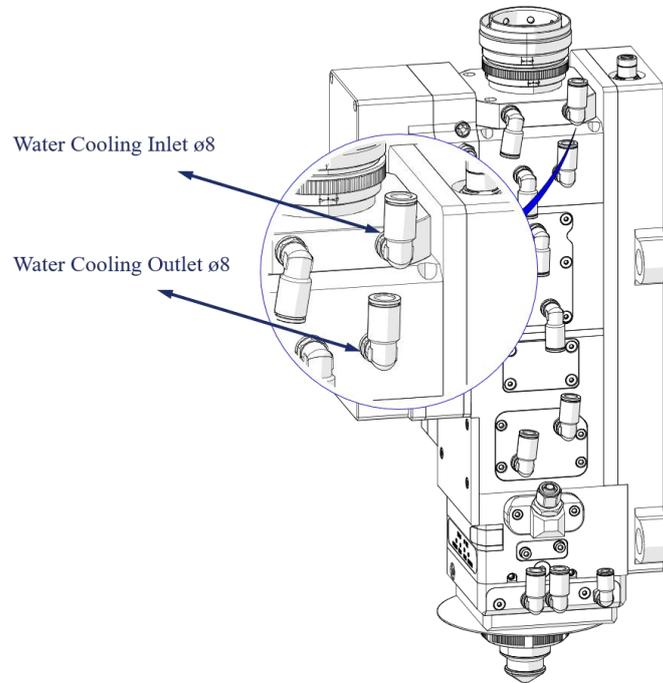
Figure 3-1 Cooling water interfaces
