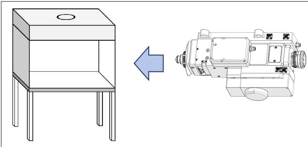
Figure 5-3 Put the cutting head inside the workbench
