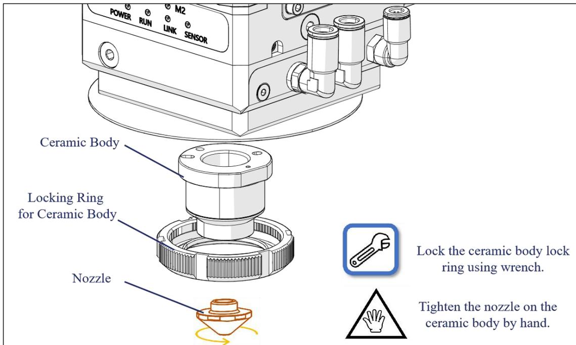
Figure 5-8 Ceramic body and nozzle installation
