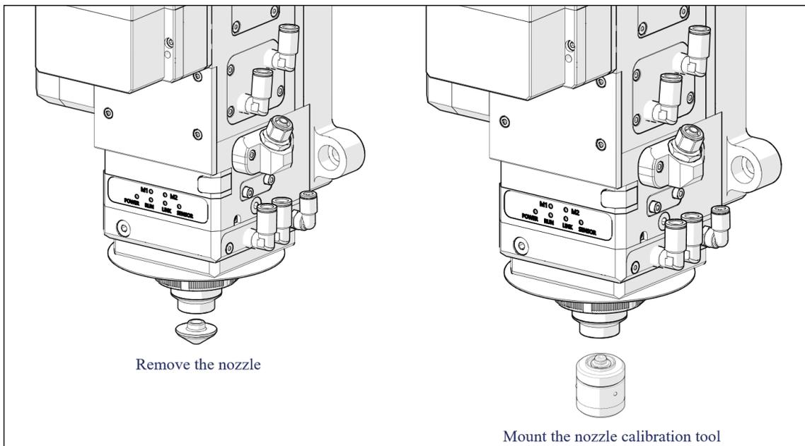
Figure 5-9 Laser beam centering
