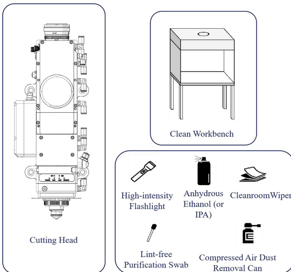
Figure 5-1 Preparation tools for the cutting head installation
