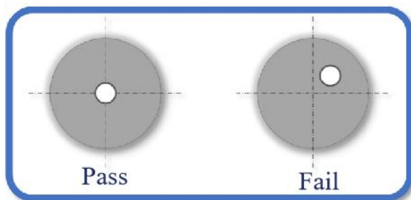
Figure 5-10 Relative position of laser beam
