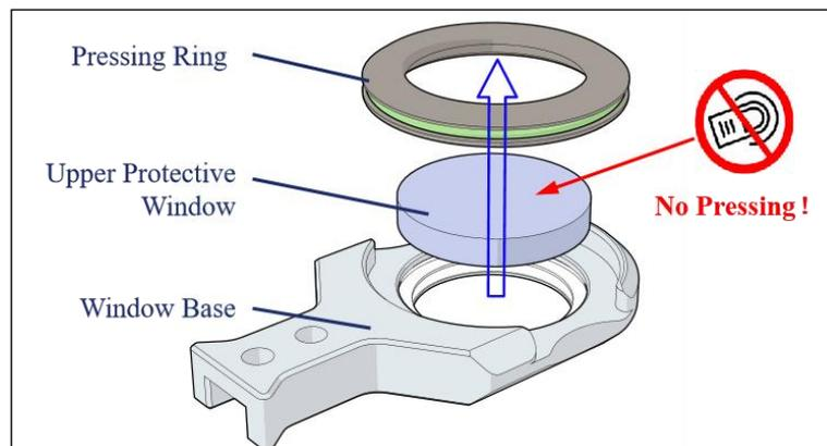
Figure 6-3 Insert window cartridge
