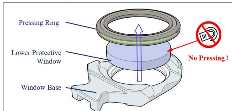
Figure 6-5 Insert window cartridge
