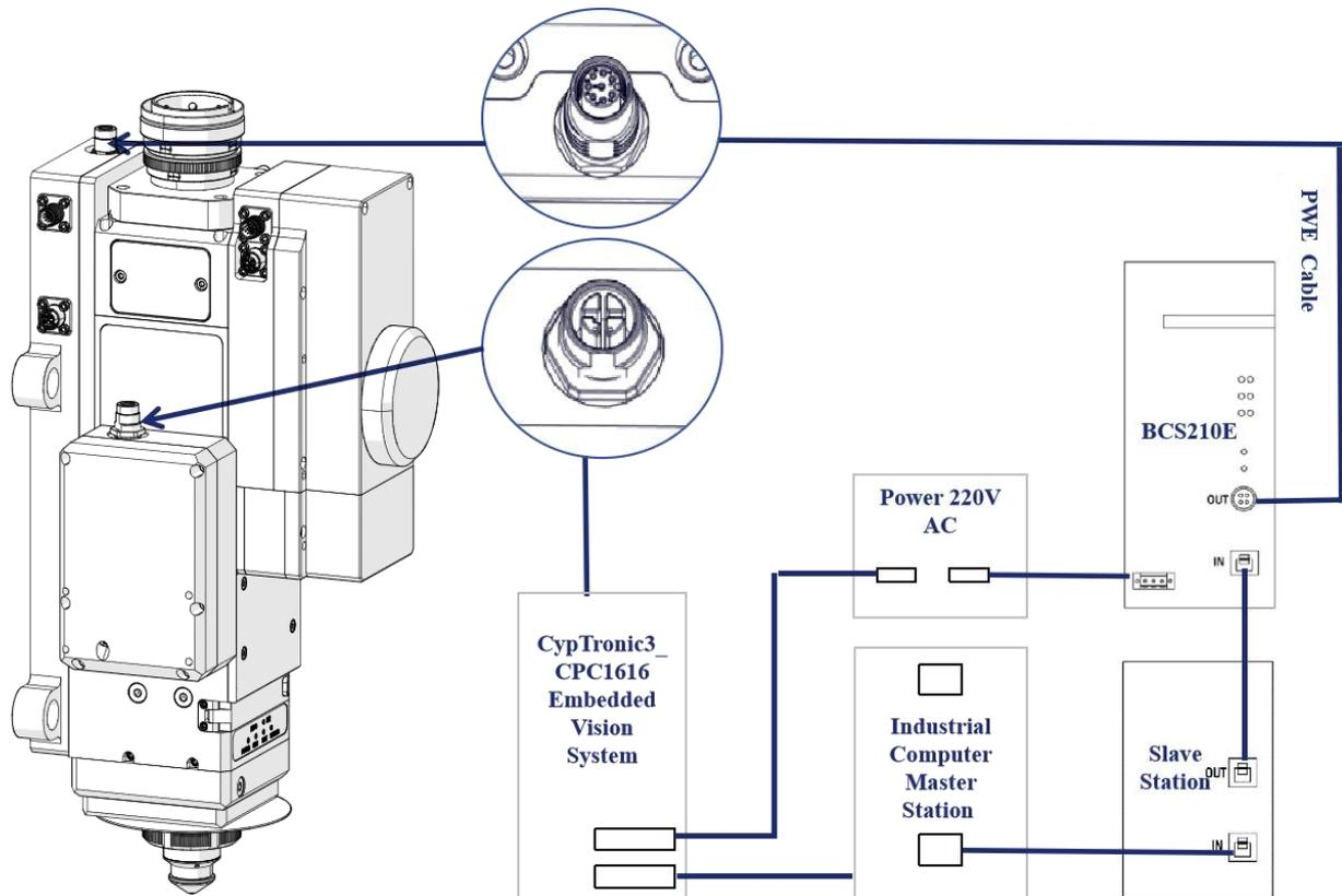
Figure 4-1 Electrical interfaces
