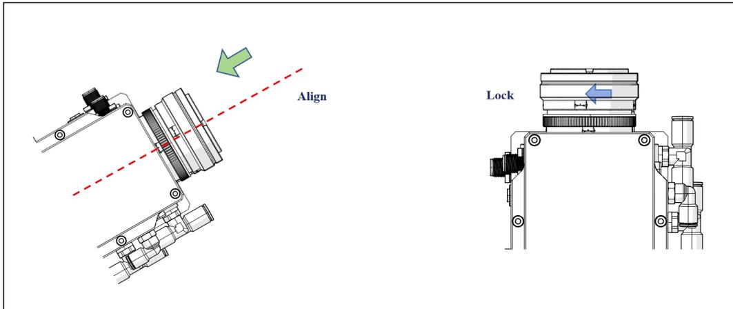
Figure 5-5 Insert the laser fiber connector
