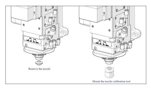
Figure 5-9 Laser beam centering
