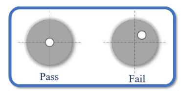
Figure 5-10 Relative position of laser beam
