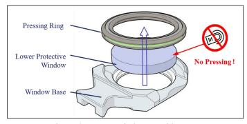
Figure 6-5 Insert window cartridge
