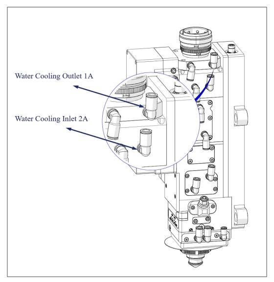
Figure 3-1 Cooling water interfaces
