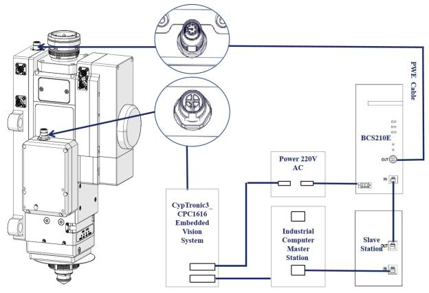
Figure 4-1 Electrical interfaces
