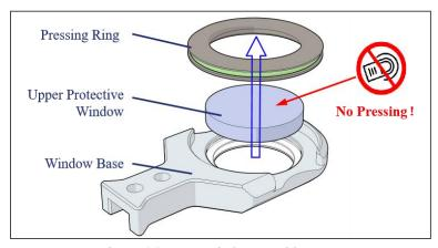
Figure 6-3 Insert window cartridge
