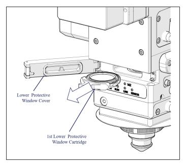
Figure 6-4 Replace the 1st lower protective window
