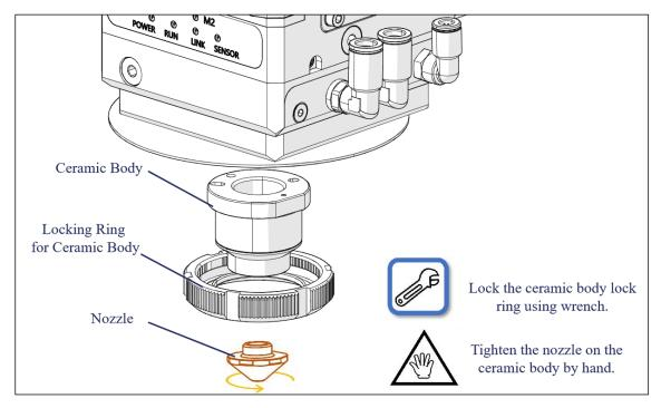
Figure 5-8 Ceramic body and nozzle installation
