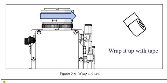
Caution: To ensure a proper seal, it is recommended to wrap at least three layers of tape for sealing.
