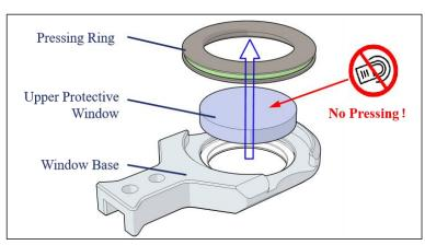
Figure 6-3 Insert window cartridge
