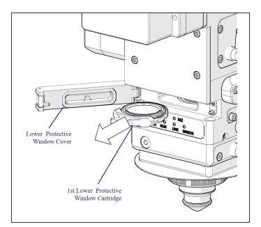
Figure 6-4 Replace the 1st lower protective window
