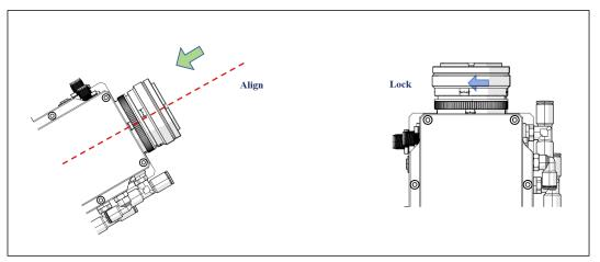
Figure 5-5 Insert the laser fiber connector
