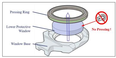
Figure 6-5 Insert window cartridge
