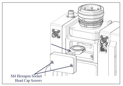
Figure 6-2 Replace the 1st protective window
