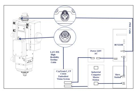
Figure 4-1 The electrical interfaces of the cutting head
