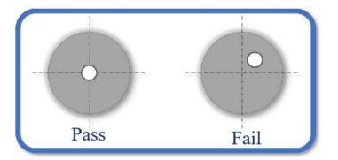
Figure 5-10 Relative position of laser beam
