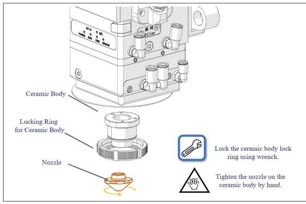
Install the ceramic body and secure it with the locking ring, then install the nozzle.
