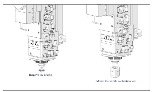
Figure 5-9 Laser beam centering
