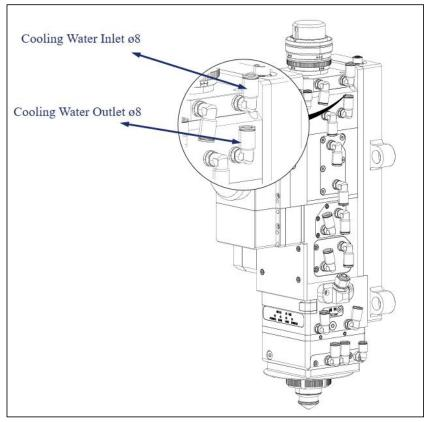
Figure 3-1 Cooling water interfaces
