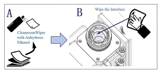
Clean the fiber interface with the cleanroom wiper soaked in anhydrous ethanol.
