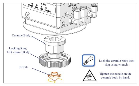
Figure 5-8 Ceramic body and nozzle installation
