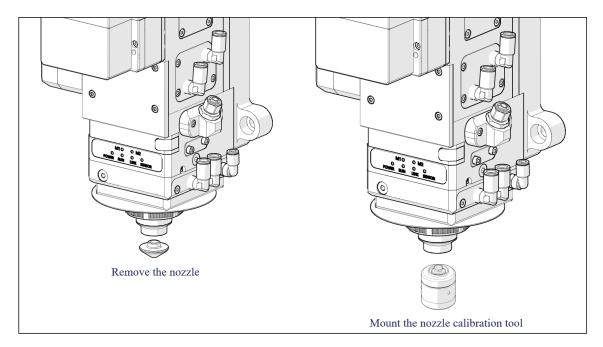
Figure 5-9 Laser beam centering
