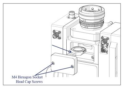
Figure 6-2 Replace the 1st upper protective window
