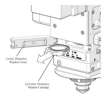
Figure 6-4 Replace the 1st lower protective window
