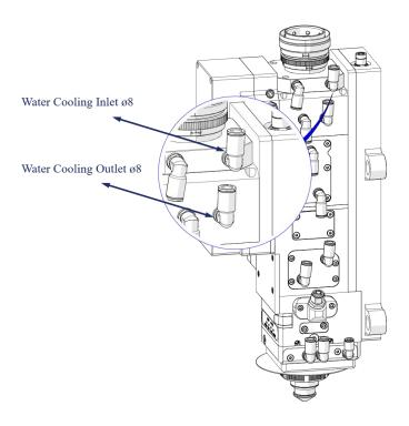
Figure 3-1 Cooling water interfaces
