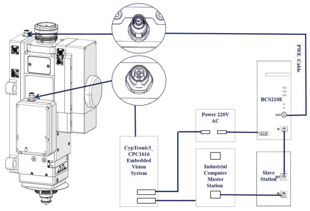
Figure 4-1 Electrical interfaces
