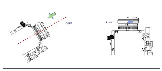
Figure 5-5 Insert the laser fiber connector
