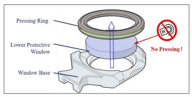
Figure 6-5 Insert window cartridge
