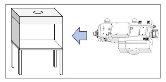
Figure 5-3 Put the cutting head inside the workbench
