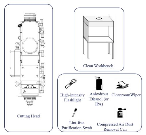
Figure 5-1 Preparation tools for the cutting head installation
