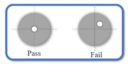
Figure 5-10 Relative position of laser beam
