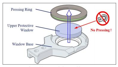
Figure 6-3 Insert window cartridge
