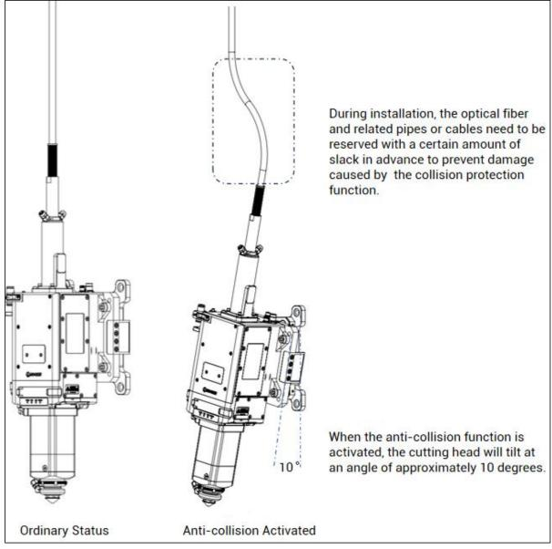
Figure 6-11 Cutting head and optical fiber status after collision
