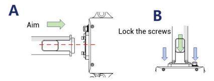
Figure 6-6 Insert the ADD fiber connector
