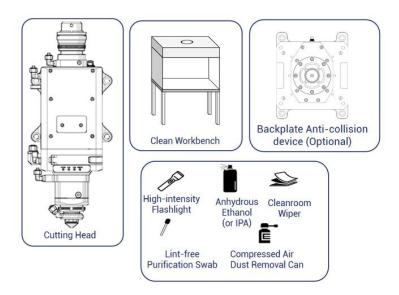
Figure 6-1 Preparation tools for the cutting head installation
