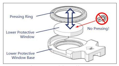
Figure 7-5 Insert window cartridge
