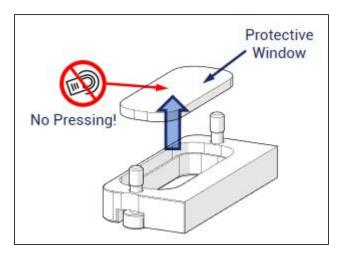
Figure 7-9 Take out the contaminated window
