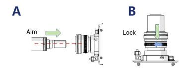
Figure 6-5 Insert the Q+ fiber connector
