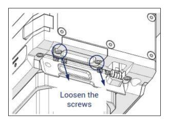
Figure 7-8 Loosen the screws
