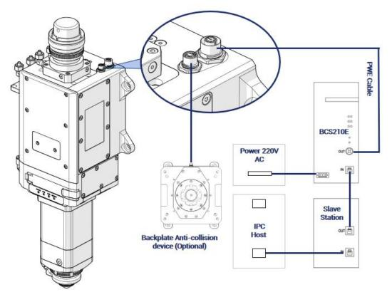
Figure 4-2 The electrical connections of the cutting head
