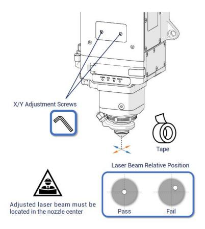
Figure 6-13 Laser beam centering
