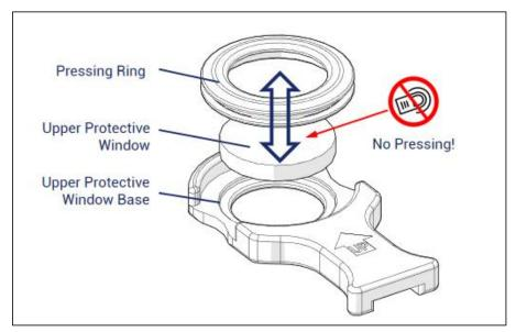
Figure 7-3 Insert window cartridge
