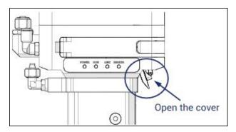
Figure 7-7 Open the cover plate
