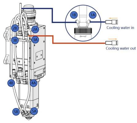
Figure 3-1 Cooling water interfaces
