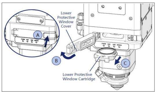
Figure 7-4 Change the lower protective window
