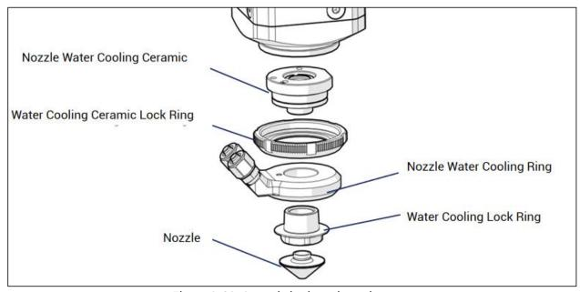
Figure 6-12 Ceramic body and nozzle
