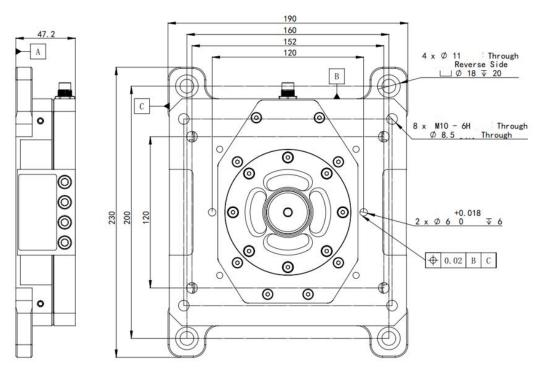
Figure 8-3 Anti-collision backplate
