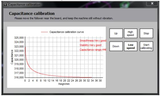
The calibration results show that the smoothness and stability are excellent indicate calibration is successful.
