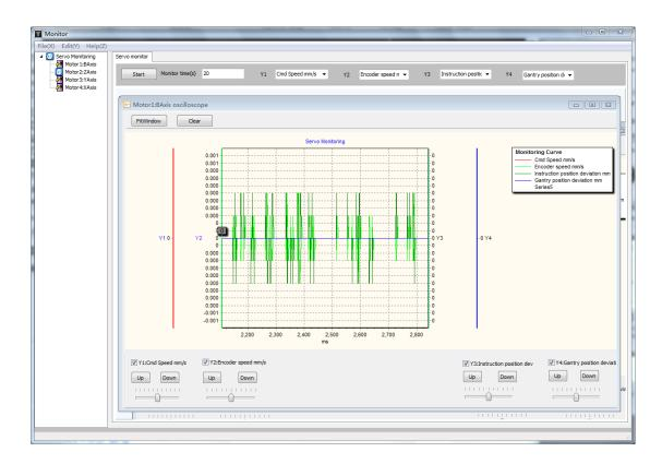
You can move mouse wheel to zoom the vertical axis of the curve. Right click to set the time range and drag to zoom view the horizontal axis. Hold the right button and left-drag the mouse to recover the graphic to proper window.
