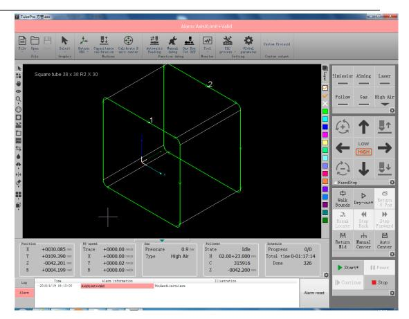
You can check the X axis status by Tool menu - > Motion control monitoring, current Limit+ is on.
