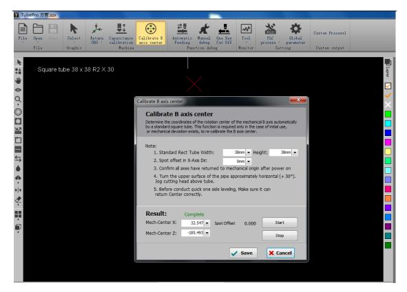
Notice: It requires accurate and reliable X/Z/B axis coordinates before calibrate B axis center, which means you need to execute Return ORG to every single axis then load and clamp the tube material and calibrate B axis center.
