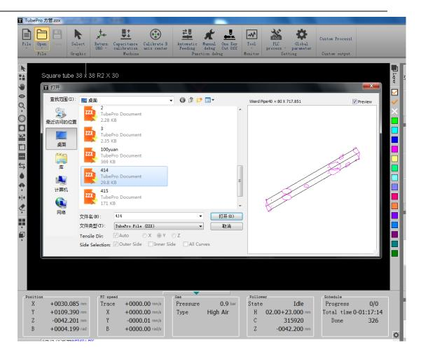
Then you can quick-set the start point, lead-in line, mid-point with CAD left tool bar and set the graphic layer and layer parameters on the right side tool.
