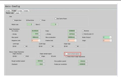
Figure 4-66 Using Z-Phase Signal
