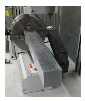
Figure 2-6 B-axis Center Calibration
