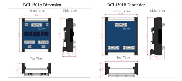
BCL1501A served to switch controlled motor axes and limit signals along with. It has three motor axes ports, three limit input ports and one control port. Within among three motor axes ports, one connected with the servo control port on main I/O board and the other two connected with servo driver. 3 limit ports connected with main I/O board and limit inputs of each axes accordingly. Control port accepts 24V DC power supply, which can realize axes switch when BCL1501A power-on.
