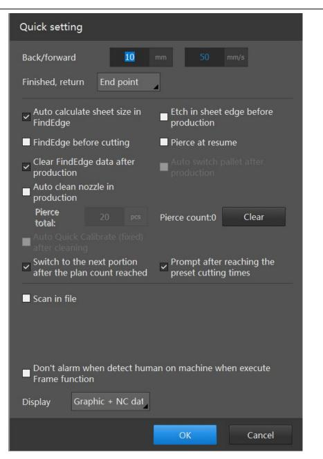
Forward/Backward: After resume from pause position, cutting path will move backward or forward by this setting then start cutting;
