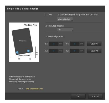
Manually move the cutting head to the edge of the plate, and record the coordinates of two different points on each edge of the plate respectively, and the system will automatically calculate the tilt angle of the plate. The longer the distance between two points is, the more precise the angle calculated is.
