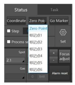
Users can set any coordinate in machine area as mark point to fast move cutter to specified position.
