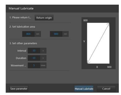
In Flexible Production and Batch Production modes, when the processing system is paused or stopped without warning, the manual lubrication button can be found in the drop-down menu of the Assist, and click to enter the manual lubrication screen.
