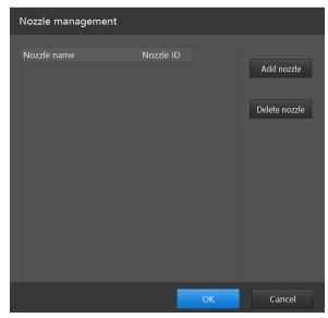
Name the corresponding nozzle and select the slot ID, then click OK to return to the Replace nozzle screen, click Nozzle Setting to configure the nozzle slot according to the actual situation. For example, if the actual nozzle replace stage is in a  $1 \times 8$  configuration as shown, set the number of rows to 1 and the number of columns to 8.
