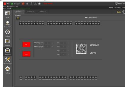
The "Limit signal' is used to show if the cutting head has reach the limit, the 'PWM' is used to show if the laser is on or off, and also shows if the other 20 inputs and 27 outputs valid.
