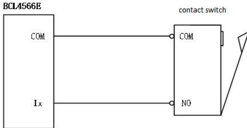
The typical connection of the magnetic induction input switch is shown in the figure below. An NPN 24V magnetic induction switch should be used.
