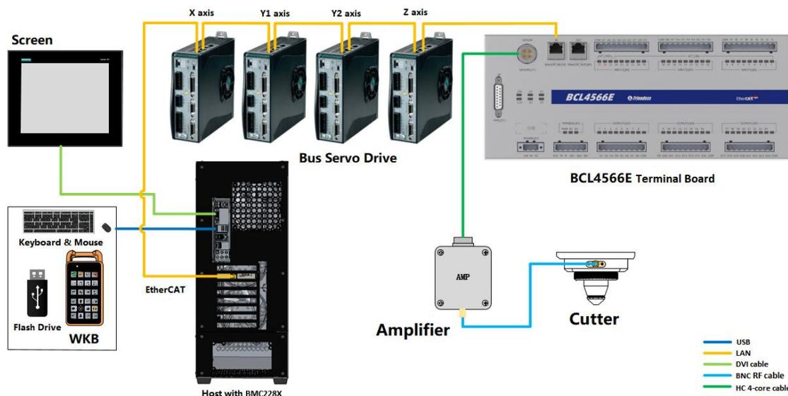
Figure 2 Wiring diagram of FSCUT2000E - non-BLT cutter
