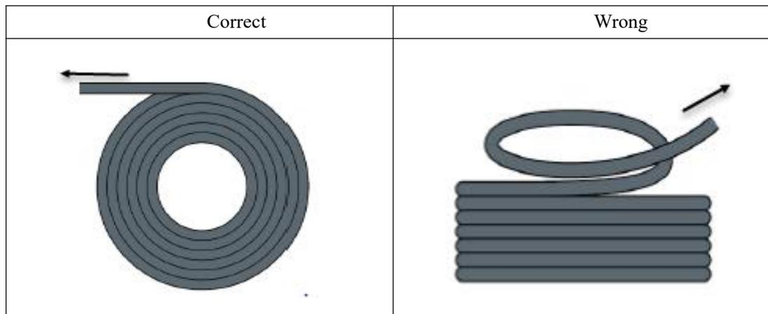
2. Cables are not allowed to be twisted when installed in a closed space, and twisting during installation may cause damage to the core wire stranding. This effect is gradually strengthened during the operation of the cable, resulting in back-twisting, which eventually leads to the breakage of the core wire and failure.
