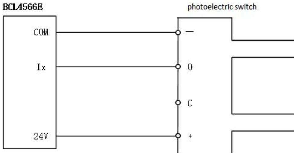
The typical connection of the contact switch is shown in the figure below.
