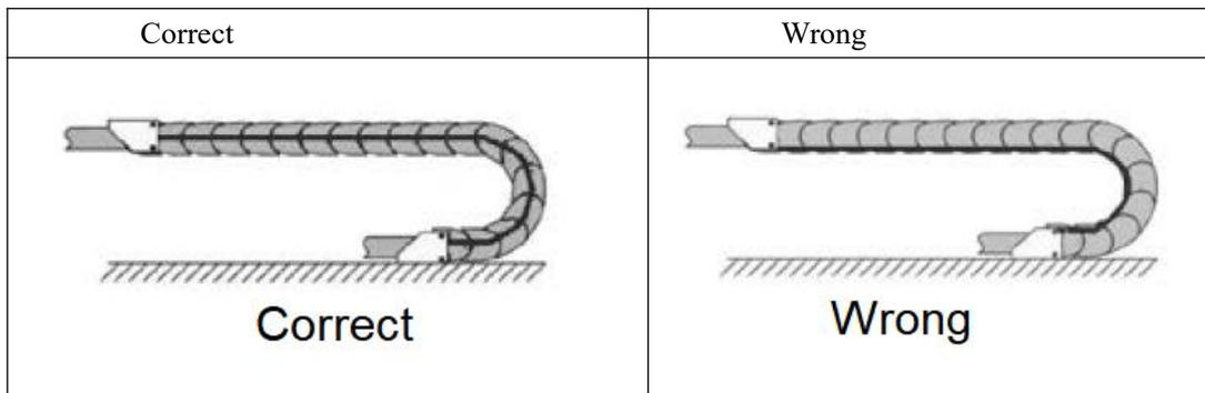
9. If the cable does not run smoothly, check whether it is twisted along the longitudinal axis during operation. The cable should slowly rotate at a certain fixed point until it runs freely.
