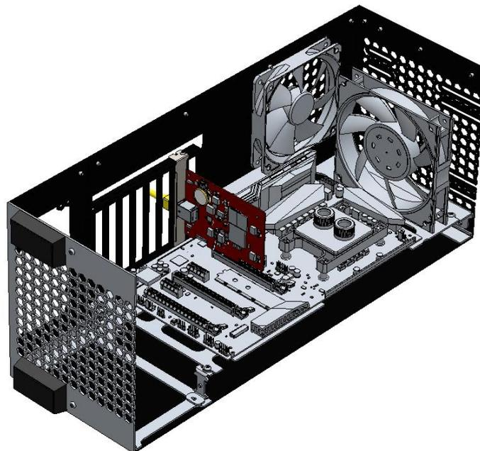
Figure 5 BMC228A Control Card After Installation
